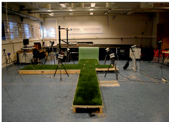
Figure 5. Left: picture of the laboratory setup. Right: schematic of the dimensions of the laboratory setup. The force plate (dark gray, 0.6 x 1.2 m) is surrounded by running tracks (light gray), with six cameras (c) angled toward the designated contact area (x). Horizontal dotted lines represent photo cell trigger beams. Dashed line arrows represent movement directions of running tasks: a straight sprint with a sudden stop (1) and a sprint with a 90° cut to the left (2).
