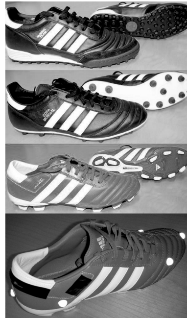
Figure 3. Cleat configurations included in the experiment. From the top: Turf cleats (adidas Mundial Team TF); Traditional round cleats (adidas Copa Mundial FG); Bladed cleats (adidas adiPURE 3 TRX FG); Placement of reflective markers on shoe (pictured: adidas adiPURE 3 TRX FG). All markers were placed at 5 cm height: one at the heel, one at the toe, and four bilaterally 6 cm in from both heel and toe. Note: sixth marker (back left side) not visible in photograph.
