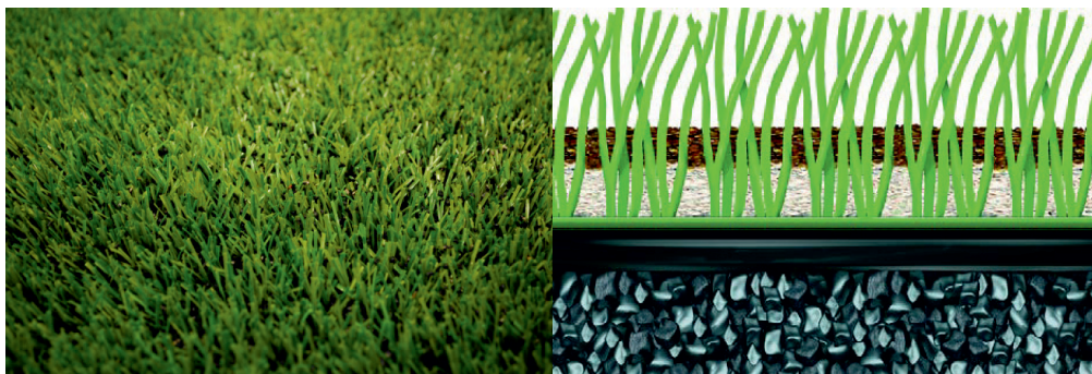
Figure 2. Left: surface view of a 3G turf system. Right: cross-section illustration of a 3G turf system (FIFA 2011a). From the bottom: foundation, leveling layer, carpet with turf fibers, sand infill, rubber infill.
