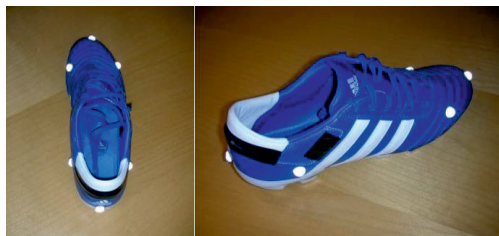
Figure 7. Placement of reflective markers on shoe (pictured: adidas adiPURE 3 TRX FG).
