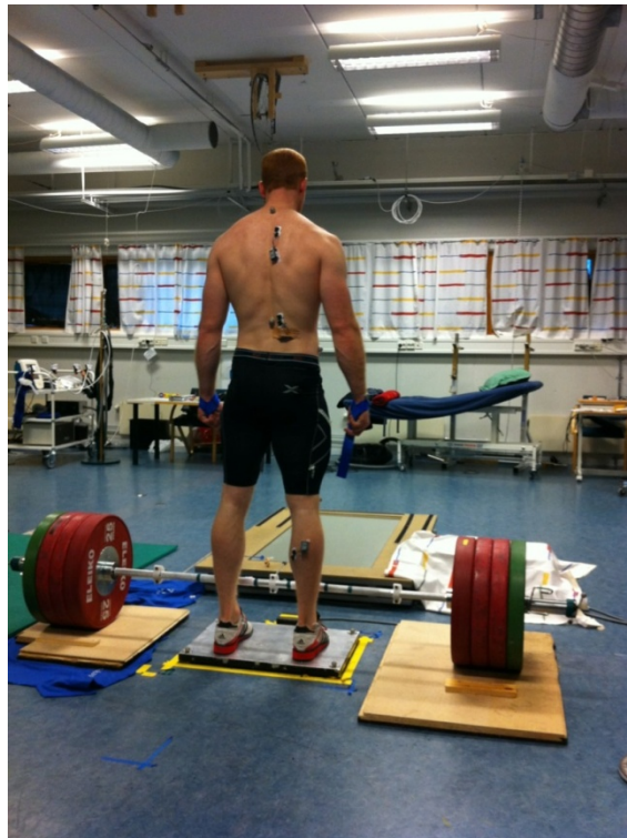
Picture 1 – Subject standing still on the force plate, ProReflex and EMG-electrodes placed on and are ready to performing the deadlift.
