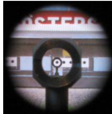
Fig 3. The picture shows the “front sight” on a biathlon rifle. The small circle in the middle is called “aperture” and was removed from the front sight. The laser dot was adjusted to be in the middle of the aiming picture instead of the “aperture”.
