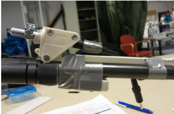
Fig 2. The laser pen and accelerometer attached at the front of the barrel
