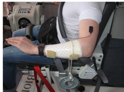
Fig 4. Setup for motor-control tasks. Arms in 45° abduction. Accelerometer placed laterally on the overarm, weights hanging proximal to the radiohumeral joint..
