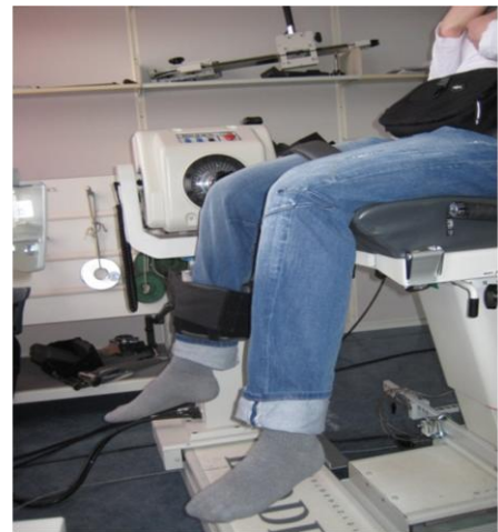
Fig 2. Setup for knee-extension MVC. The dominant leg was fastened to an attachment in a dynamometer.
