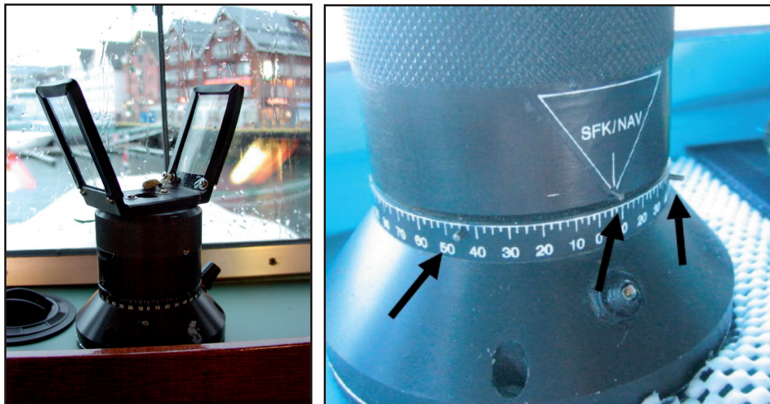
Figure 5: The optical bearing device. The three alignment pins and the scale can be seen on the close up picture to the left. Photo by the author.
