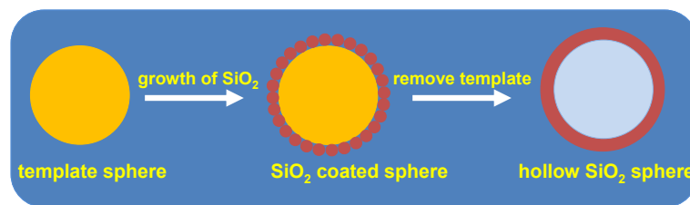
Figure 1. Illustration of the synthesis process when fabricating hollow silica nanospheres (HSNS) by the sacrificial template method.
