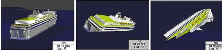
Figure 1.1: Sequence of events in the sinking of MV Estonia (image from final Accident Investigation Commission report, 1997)
