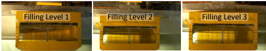
Figure 2.3: Damaged section in forced heave motion at three filling levels
