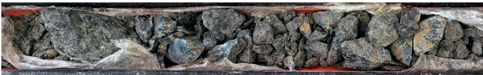
Fig. 2 Serpentinite rock extracted from the borehole drilled parallel to Headrace tunnel at Moglicë HPP
