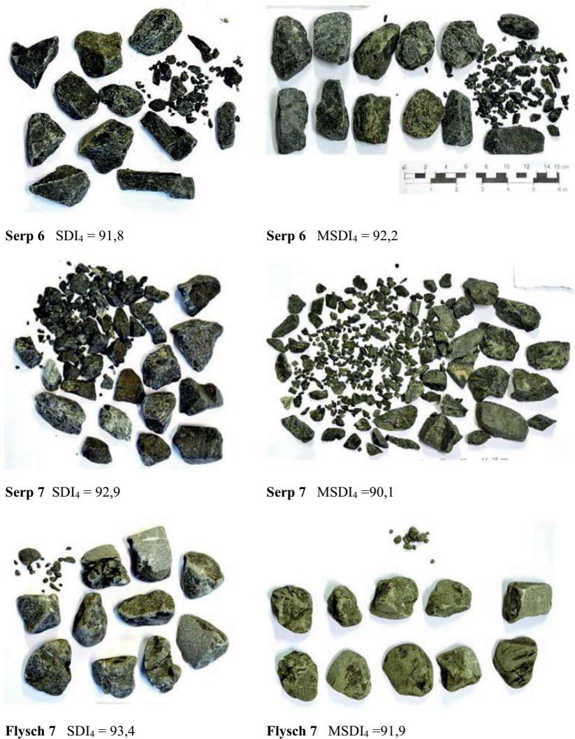
Fig. 12 Samples showing similar slake durability indices but different disintegration behavior
