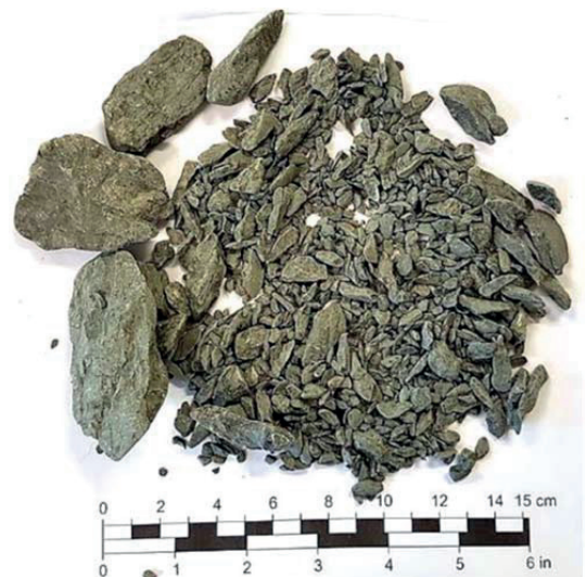
Fig. 11 Splintered material of Flysch 11 after the ISRM slake test
