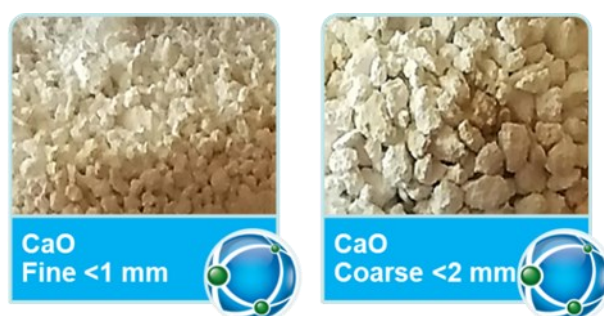
Figure 5. Physical appearance of fine CaO to the left and coarse CaO to the right.
