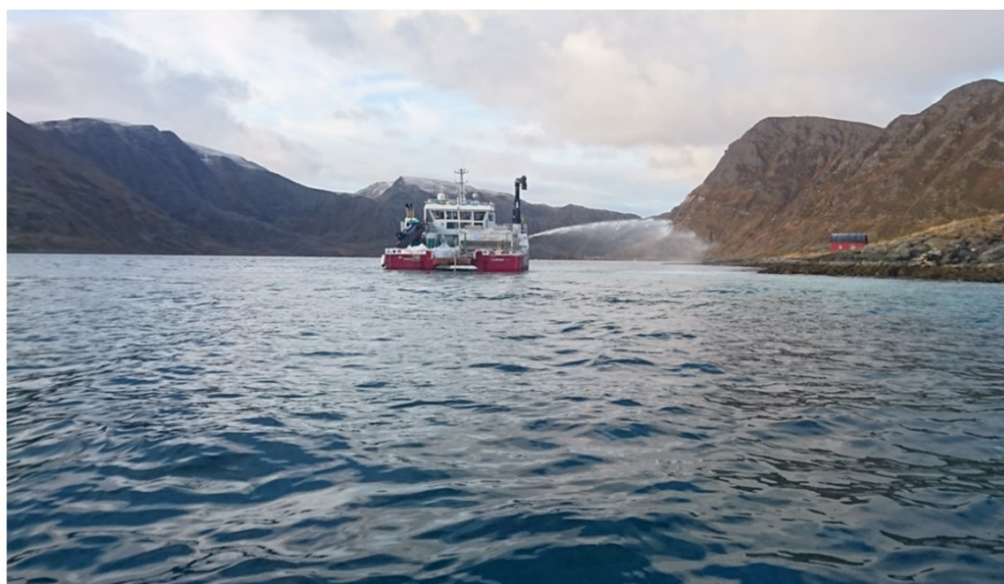
Figure 18. Photo of the boat spraying lime suspension of coarse CaO over the sea.
