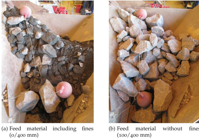
Figure 3.2: Examples of photos used in digital image processing of feed particle size distributions. Photo: Metso Minerals
