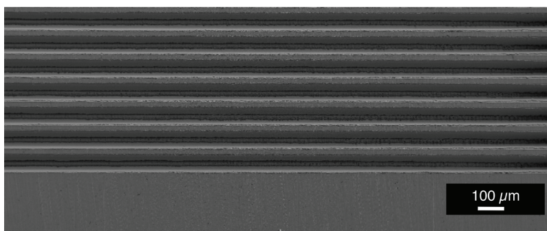
Fig. 2. SEM micrograph showing example top view of the equidistant lines produced by laser structuring steel surfaces with a periodic pattern of peaks. Sample B2 is shown here.
