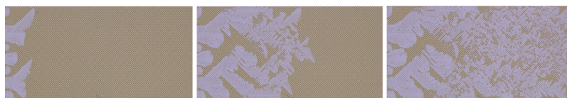
Figure 7. Crude oil A displaced by HS-Na at 5 \mu\text{L}/\text{min} at 5, 15, and 25 s (breakthrough).
