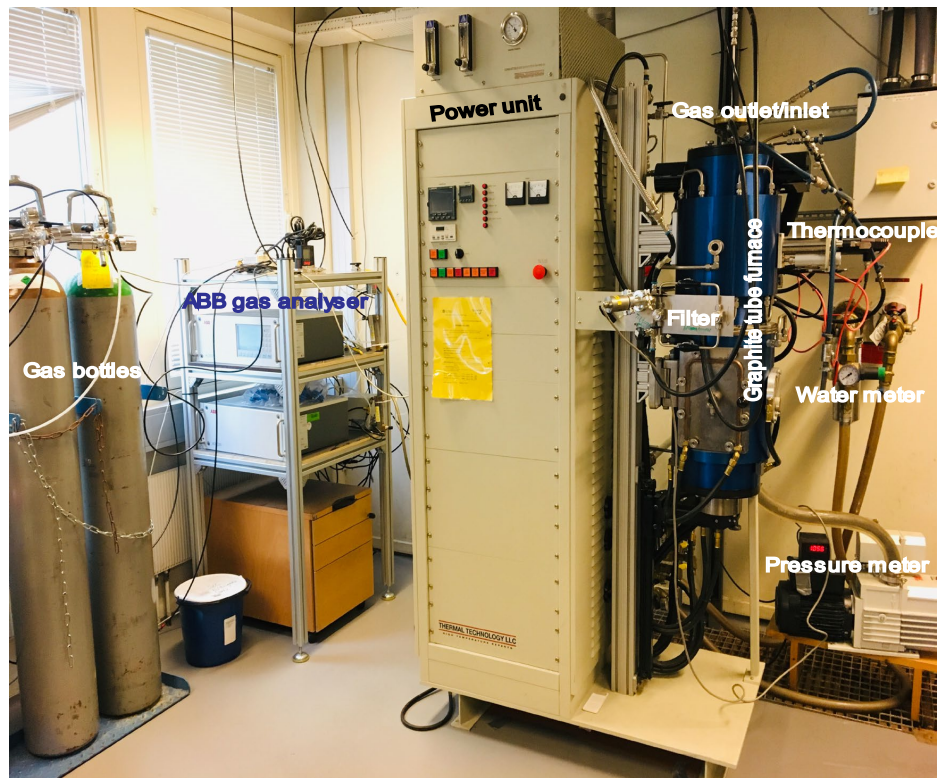
Figure 3.3.10. Graphite tube furnace (Thermal Technology Model 1000-3560-FP20).
