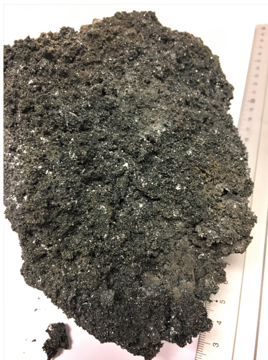
Figure 4.4.1. SiC-ELT obtained from Elkem Thamshavn furnace 2.
