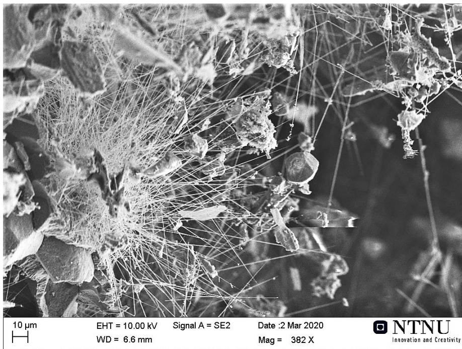
Figure 4.4.10. SEM morphology of part of SiC-ELK, close to condensate region (region A).
