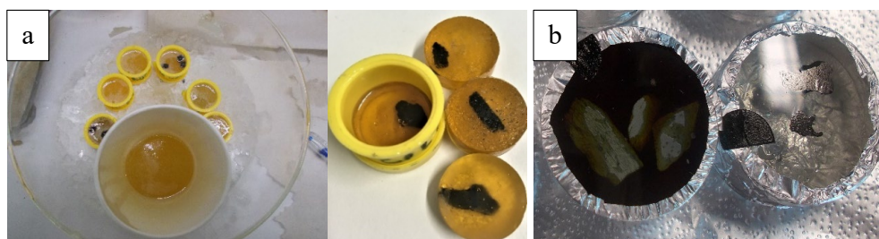
Figure 3.6.1. (a) Sample in iodoform-epoxy mixture kept for solidifying in ice bath and sample after solidification. (b) Sample in an iodoform-epoxy (left) and a normal epoxy (right).
