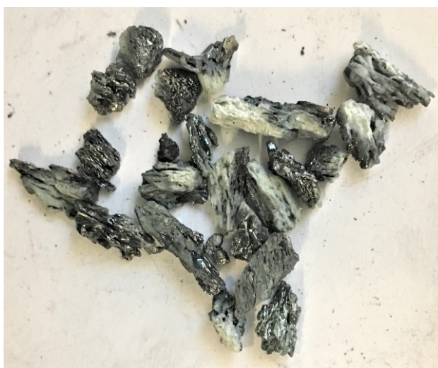
Figure 4.1.41. White and light bluish condensates observed on surfaces of particles used for filling the condensation chamber, from experiments performed with pellets of ( \text{SiO}_2 + \text{SiC} ).
