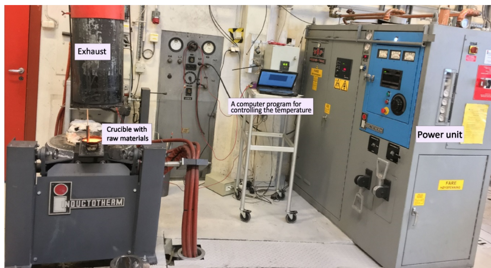
Figure 3.3.1. IF75 induction furnace used for experiments, along with power supply.
