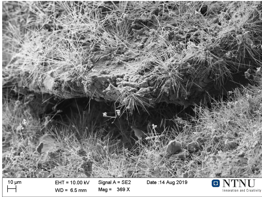
Figure 4.3.4. SEM images of SiC from middle layer, exposed to a temperature < 1750 °C. SiC crystals in the shape of whiskers have formed.
