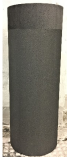
Figure 3.3.3. Graphite crucible used for \beta -SiC production in induction furnace.
