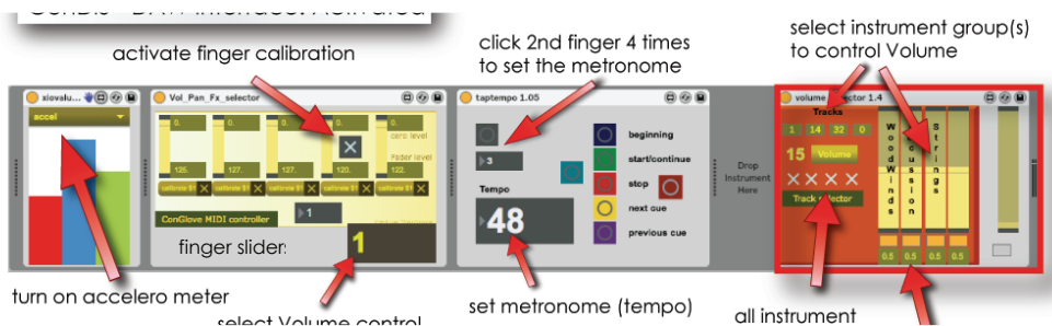
Figure 58. The ConDiS system activated. The accelerometer activated, finger calibration on, tap tempo and metronome set, and volume levels up (turned red).
