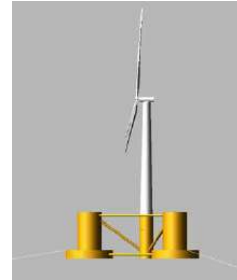
Figure 8 OC4 Semi-submersible wind turbine [21]
