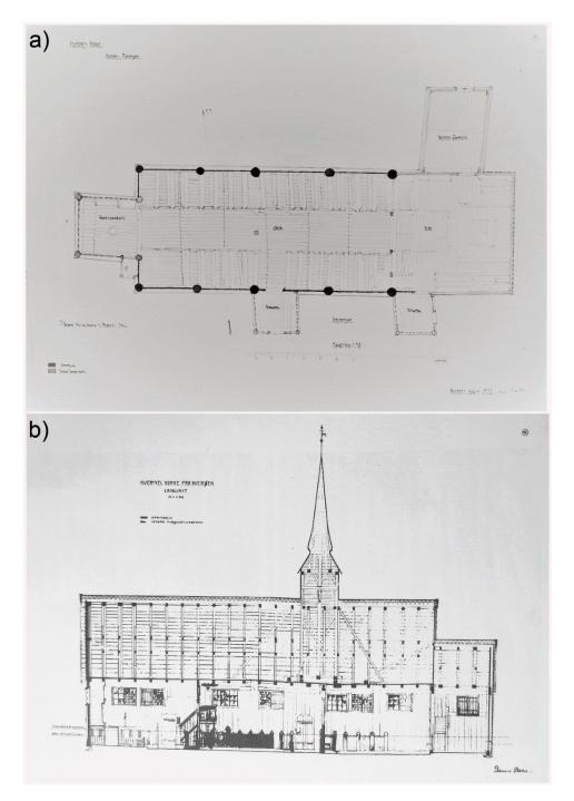
**Figure 2.** Kvernes stave church. (**a**) Planimetry; (**b**) vertical section. The south wall. Source: Illustrated guide to the stave church by the architect Heinrich Joachim Sebastian Karsten (1873–1947) in 1900.
