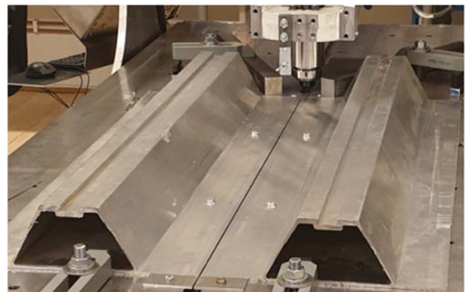
FIGURE 1 Photograph showing the experimental set-up employed in the HYB butt welding trial with the 4mm AA6082-T6 Johan Sverdrup profiles
