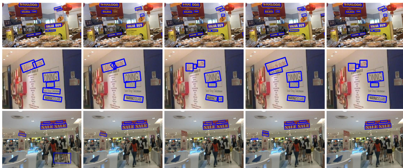
FIGURE 7. The fusion of multi-oriented bounding boxes detected by deep learning-based methods. The first four columns illustrate detection results achieved by the Pelee-Text, TextBoxes++, PixelLink, and PSNet networks, respectively, and the last column shows the performance results achieved by our GP-based fusion method.
