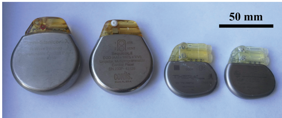
Figure 2.19: Four generations of artificial cardiac pacemakers. From left to right: Cordis' Omni-Stanacor ® , Cordis' Sequicor ® , Medtronic's Thera ® and Medtronic's Adapta ™ .
