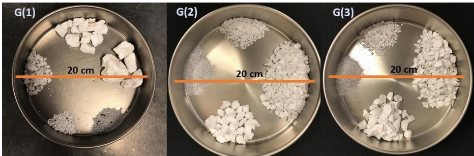
Figure 94: Quartz sample G(1), G(2) and G(3) after shock heating at 1500 °C and sieving.
