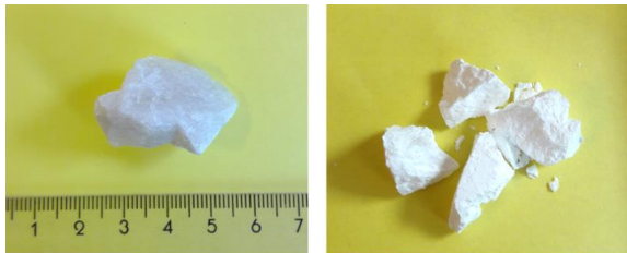
Figure 111: Sample F2 before (left) and after (right) heating 1600 °C and held for 120 minutes. The sample was 9.7 g and 2-3 cm in size.
