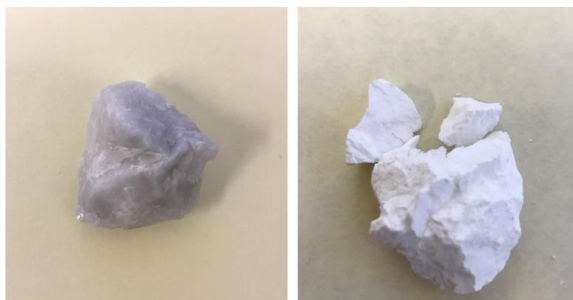
Figure 112: Sample G3 before (left) and after (right) heating to 1700 °C and held for 0 minutes. The sample were 11.0 g, and 2-3 cm in size.
