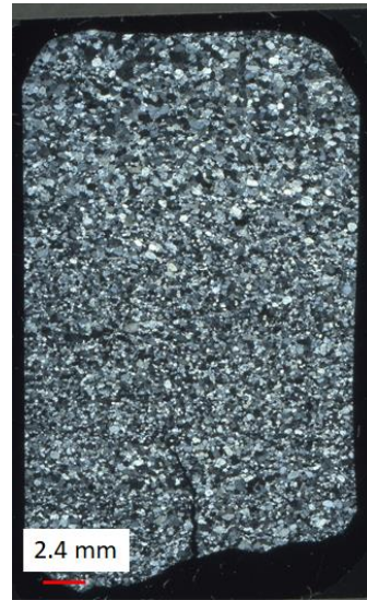
b) Thin section of quartz type D, after shock heating.
