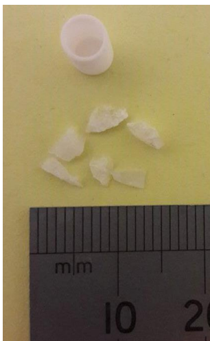
Figure 181: Quartz samples used for DTA experiments. The total sample weight for each experiment were 50-70 mg.
