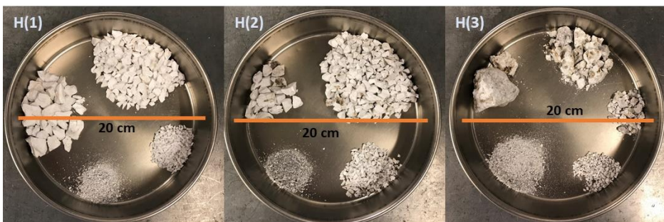
Figure 95: Quartz sample H(1), H(2) and H(3) after shock heating at 1500 °C and sieving.
