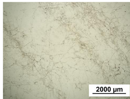
b) Fractures crossing the sample from the top left corner to the bottom right.
