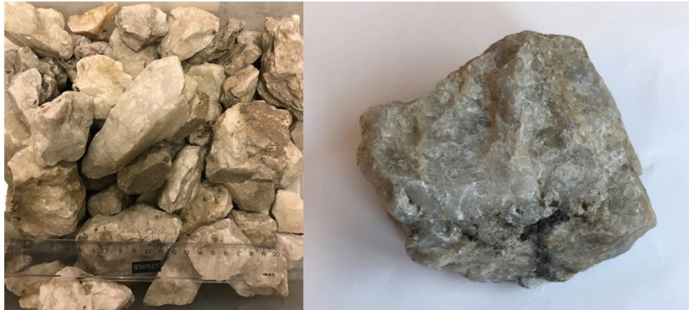
Figure 67: A batch and a separate lump of quartz type F.
