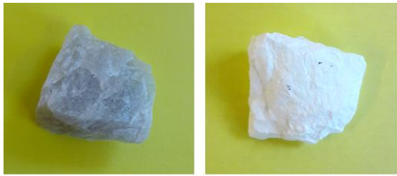
Figure 110: Sample A11 before (left) and after (right) heating to 1700 °C and held for 60 minutes. The sample were 10.8 g, and 2-3 cm in size.
