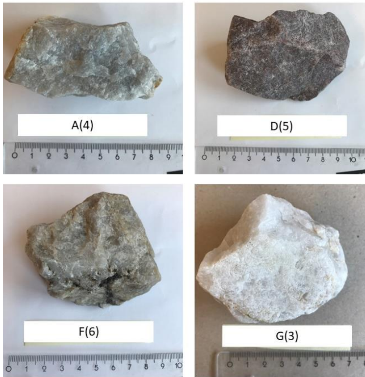
Figure 77: A sample from each of the four main quartz types shock heated. The samples were 200 g \pm 20 g and 5-9 cm in diameter.
