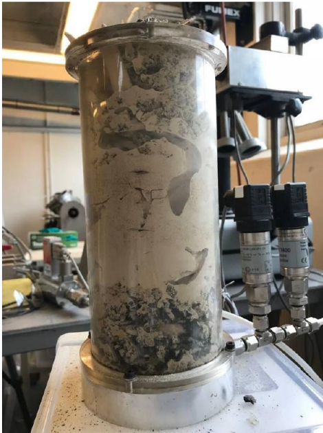
Figure 10: Channel formation in the permeability test cell with charge materials and quartz below 1 mm [15].
