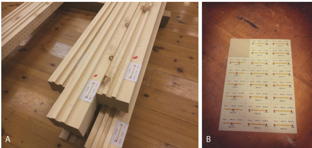
Figure 76: The output from the Grasshopper model was A4-sheets of stickers, which contained ID, position, length, and eventual holes.
