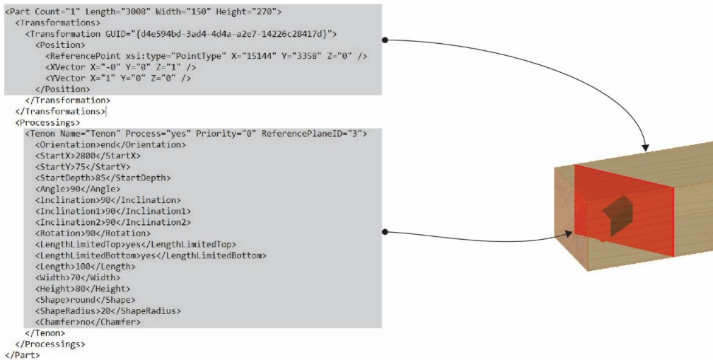
Figure 15: BTLx is XML-based. The figure shows how a blank and tenon are defined.
