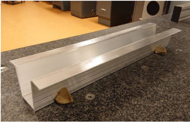
Fig. 7 Overview of profile sample located in coordinate measurement machine
