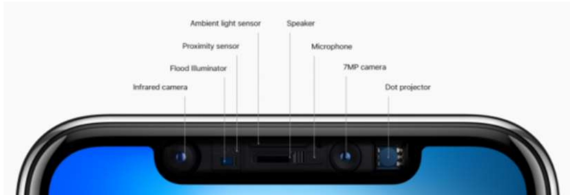
Figur 38 - Maskinvare til Apple's TrueDepth kamerasystem (Hentet fra https://www.extremetech.com/mobile/255771-apple-iphone-x-truedepth-camera-works )
