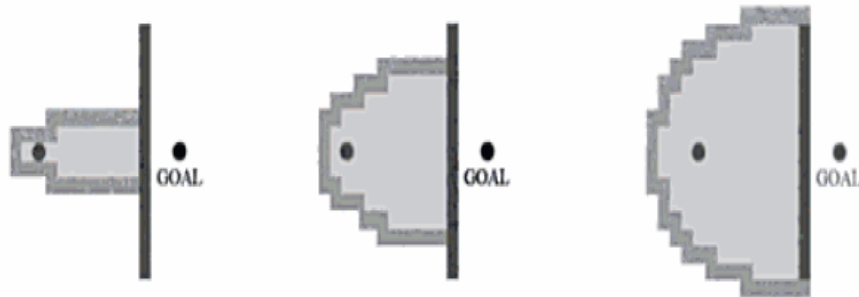
Figure 4: A* algorithm (heuristic cost using Euclidean distance)
