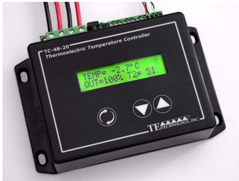
Figur 45- temperaturregulator TC-48-20 (Fra TE Technology) https://totech.com/wp-content/uploads/2013/09/tc-48-20_manual.pdf
