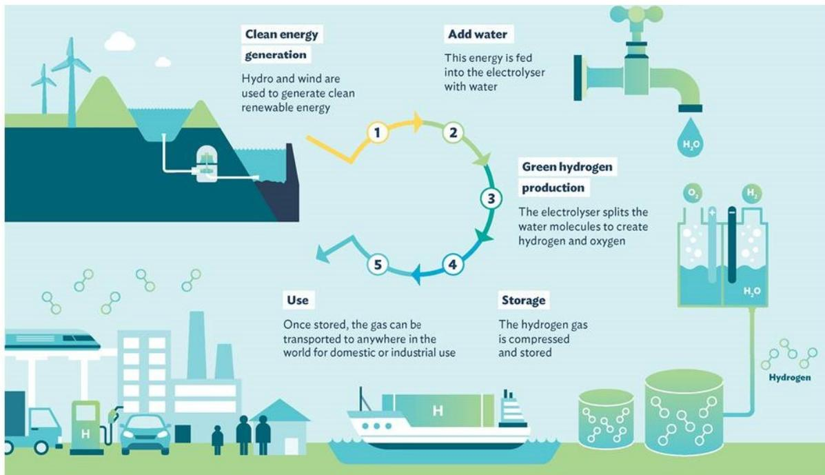
Figure 3.1: Green hydrogen produced from clean energy through water electrolysis [53]
