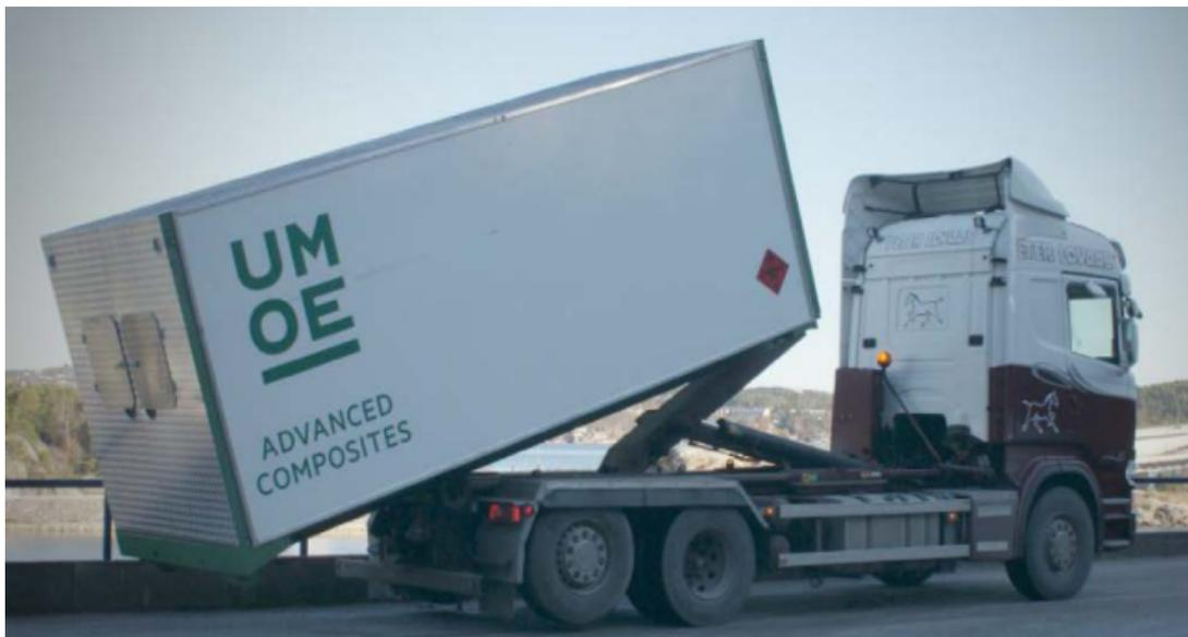
Figure 7.3: UMOE Advanced Composites container that can be lifted on top of the truck [11]
