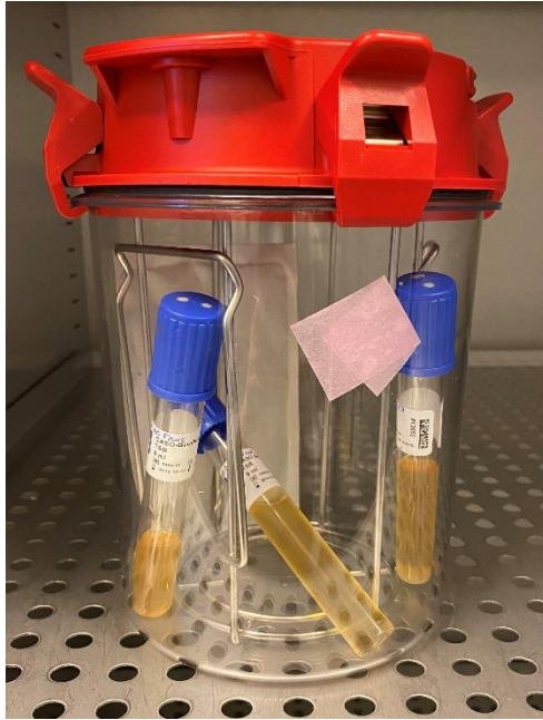
Figure 3.1: Anaerobic jar for cultivation of F. nucleatum. Anaerobic conditions were achieved by anaerobic atmosphere generation bags (white bag) and the anaerobic conditions were monitored by an anaerobic indicator test (pink patch on wall of anaerobic jar). The anaerobic indicator change color from pink to white indicating anaerobic conditions. Tryptic soy broth medium containing F. nucleatum in tubes with blue cap. F.A.A. agars were incubated in the same manner.
