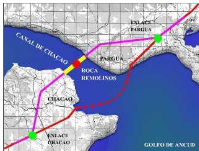
Figure 7.2: General Layout of the Chacao Channel Tunnel. This figure was originally developed as part of the feasibility study for the bridge project that is being developed. The tunnel alignment follows
