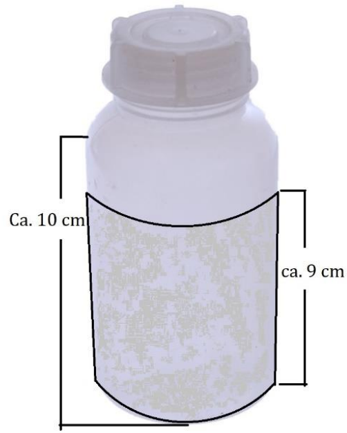
Figure 19: Test bottle with its height ca. 10 cm, and the slip height ca. 9 cm.
