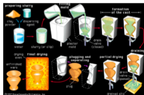
Figure 2: Slip casting process [2].
