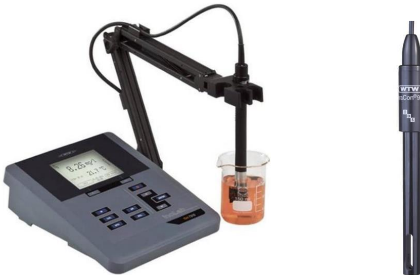
Figure 16: WTW Inolab Cond. 7110 conductivity meter (left) and its measuring cell (right) [32].
