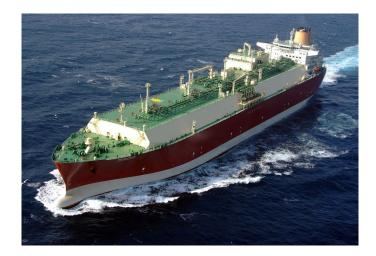
Figure 2.17: Membrane LNG tanker (Qatargas, 2013)
