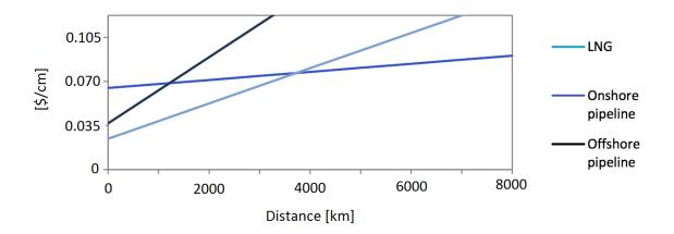
Figure 2.2: Transportation cost per cubic meter of gas as a function of distance for onshore pipeline, offshore pipeline and LNG
