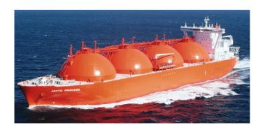
Figure 2.18: Self supporting LNG tanker (Global Security, 2013)
