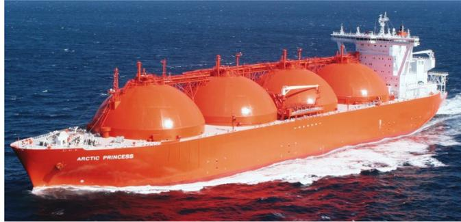
Figure 2.18: Self supporting LNG tanker
