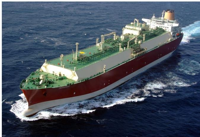
Figure 2.17: Membrane LNG tanker
