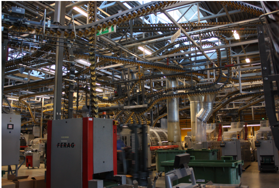
Figure 5: Gripper-conveyor system at Nydalen printing facilities
