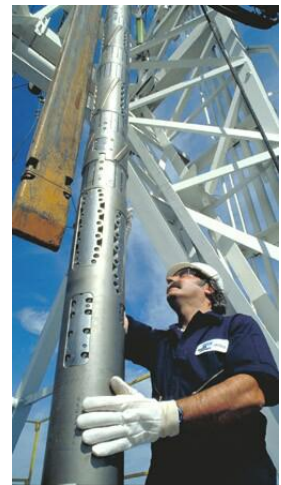
Figure 8: Well logging tool string suspended by a derrick above an oil well (IAEA, 2010)
