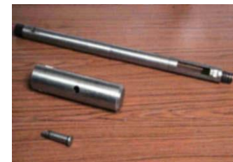
Figure 10 Gauge for measuring the density of well fluids (IAEA, 2003)
