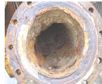
Figure 14: Left: places where NORM may accumulate in the recovery process. (OGP , 2008). Right: NORM scale inside a pipe (NET Waterjet , 2014)
