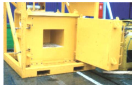
Figure 21: Transport container used as a temporary store for well logging sources (IAEA, 2003)
