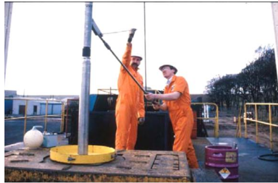
Figure 32: Wire-line engineers transferring radioactive sources to logging tools, by use of handling rod (IAEA, 2003)
