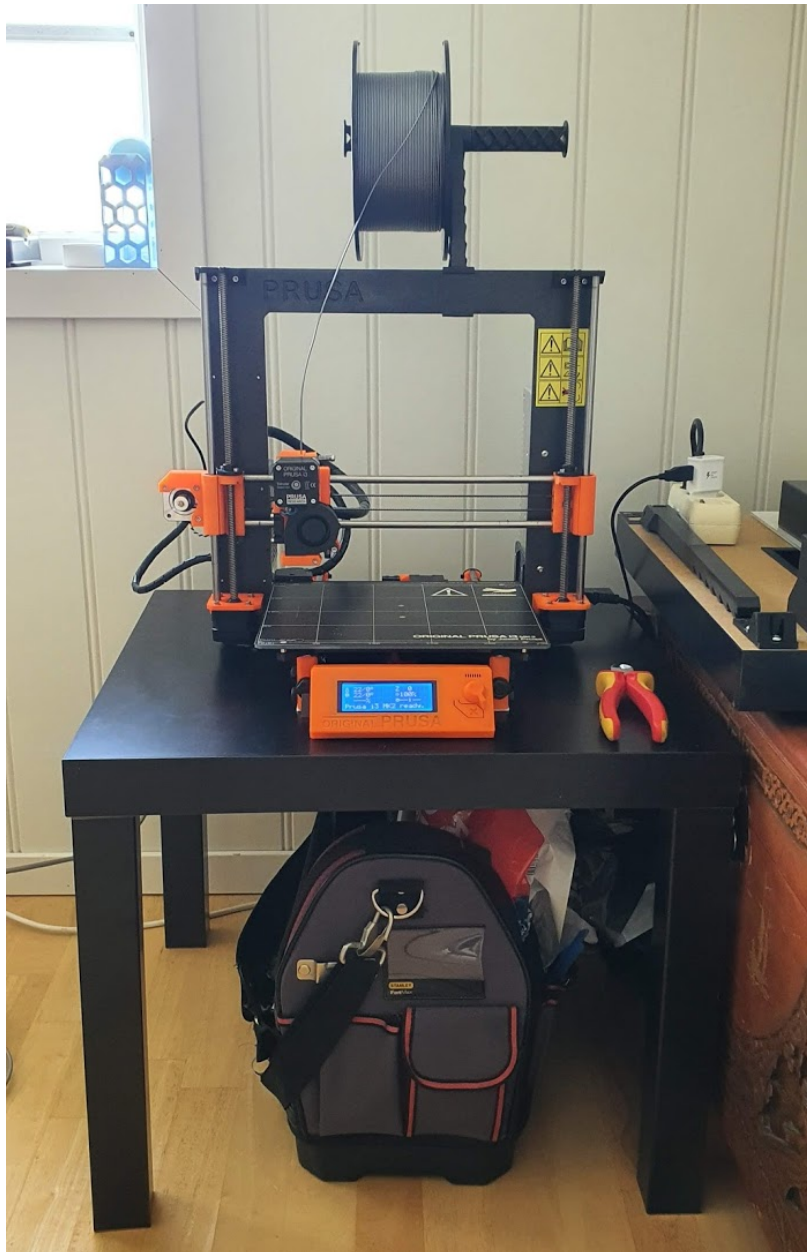
Figure 4.5: Private Prusa i3 MK2 setup used to complete printer communication. A Raspberry Pi 1 B+ is mounted to the bottom of the table.
