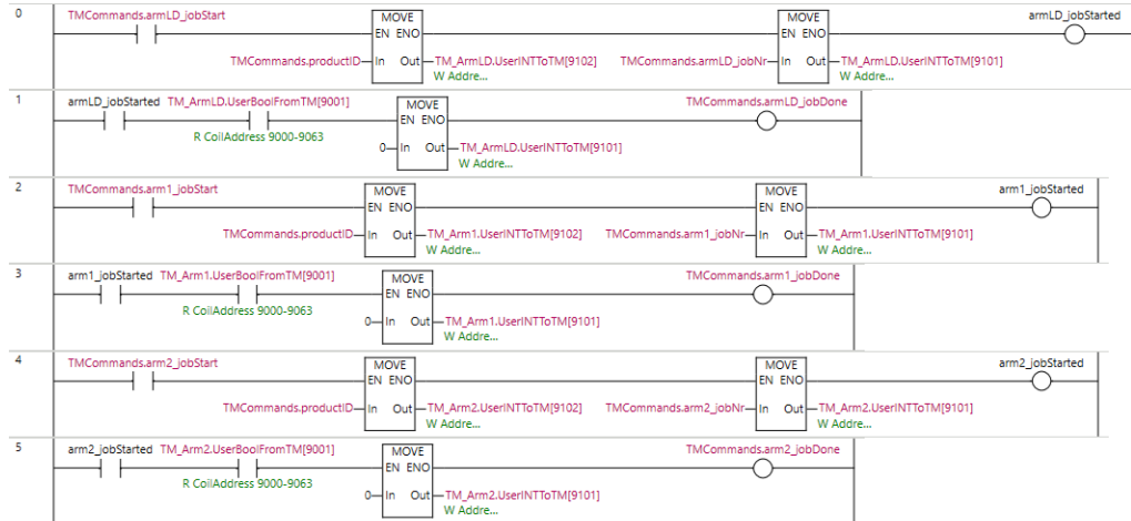
Figure 3.27: doTask function in the main program, 2 lines per TM robot arm
