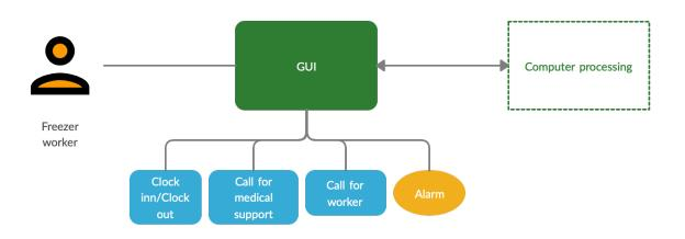
Figure 31: HMI outside freezer
