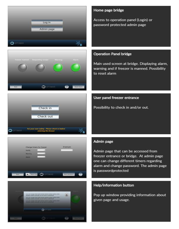
Figure 41: HMI test design 3
