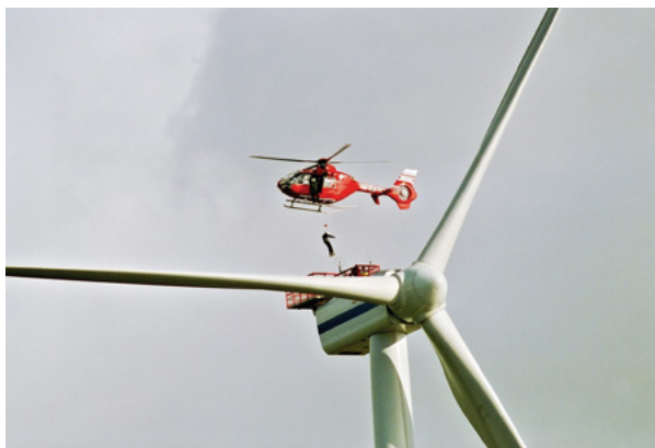
Figure 11: Engineer lowered onto the nacelle by a helicopter. Photo: Eurocopter
