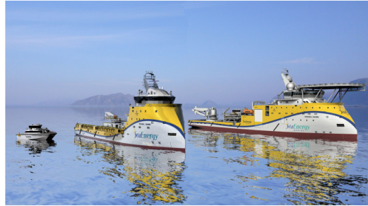
(b) Ulstein's X-bow concept. Photo: Ulstein Group
