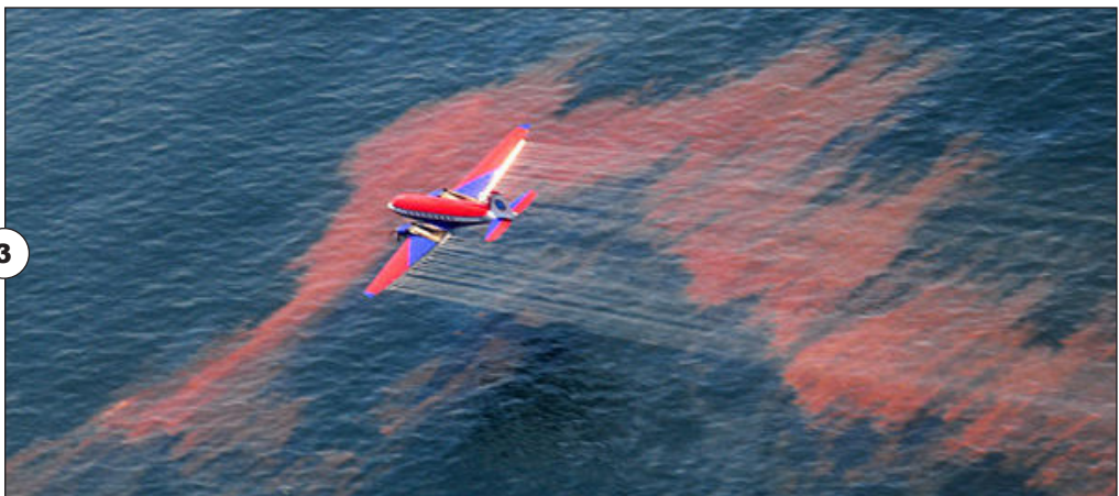
■ Figure 9: Images of OSR technologies. (1) Standard oil boom. (2) Foxtail skimmer. (3) Dispersion system mounted on an airplane. (4) Aptomar Securus system. (5) High pressure system for on-land cleanup. (6) In-situ burning of oil.
