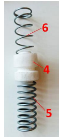
Picture 37. Dual functioning spring
