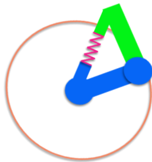
Illustration 7. Hinge with spring and lever arm
