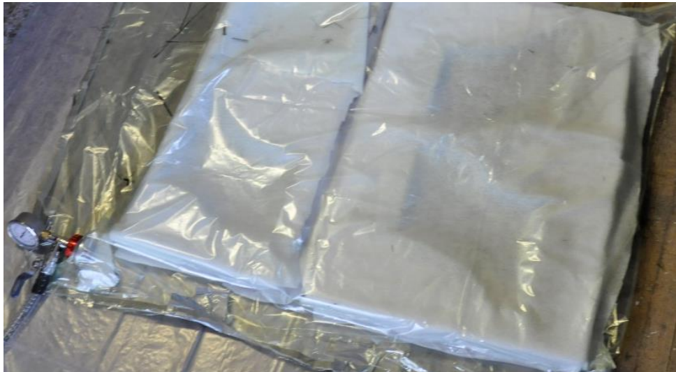
Figur 44: Former satt under delvis vakuu
