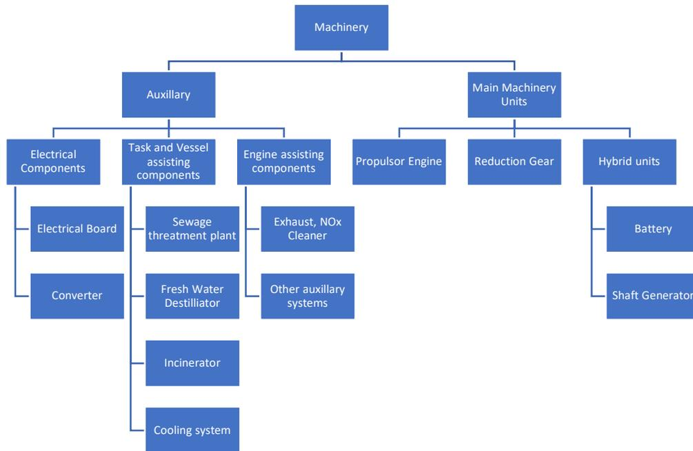
Figure 75: Machinery Main Components
