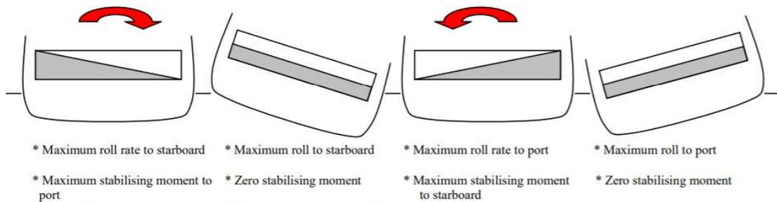
**Figure 4 Surface tank demonstrating the basic principle of passive tank roll damping.**
