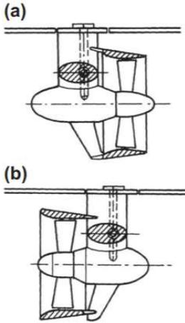
Figure 18: Azimuth thruster types (a) pushing, (b) Pulling unit, (Carlton, 2012)
