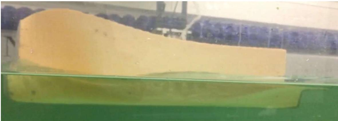
Figure 195: 14 kn Wave Profile
