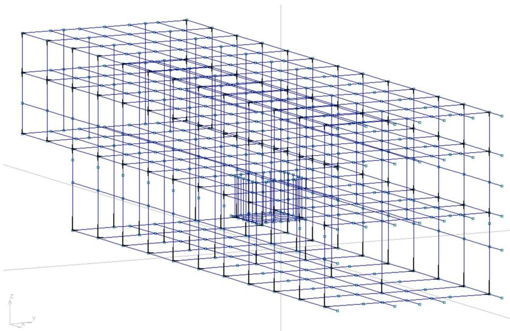
Figure 130 Structural arrangement from aft to fwd bulkhead
