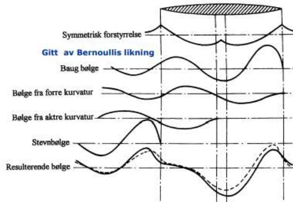
Figure 79: Wave Picture Around a Hull
