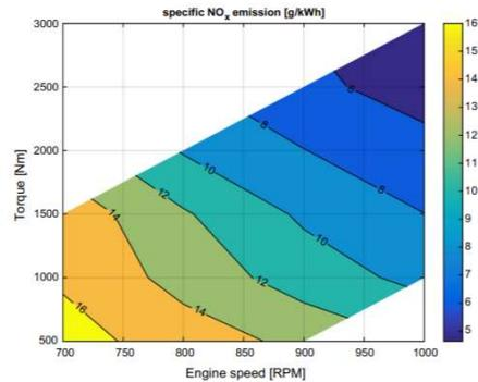
Fig. 4. NO<sub>x</sub> measurement results of MAN4L20/27 research engine on Netherlands Defence Academy in contour plot, from Linden [31].
