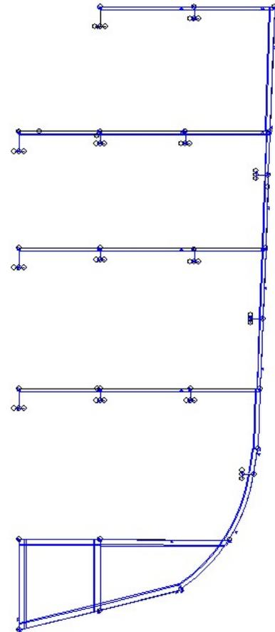
Figure 132 Section scantling model of hatch section frame #85
