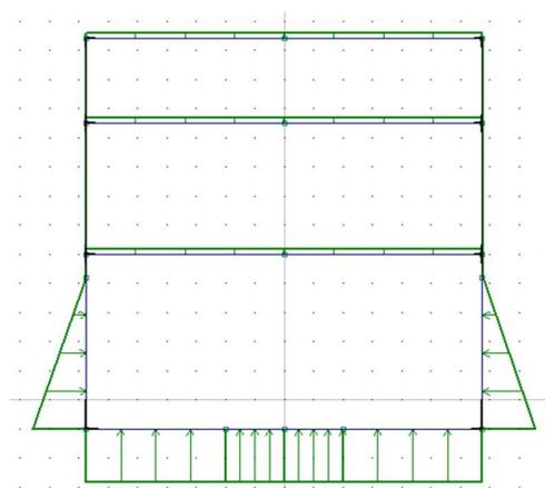
Figure 101 Load applied on a longitudinal stiffened structure. Here is only design loads and static water pressure applied
