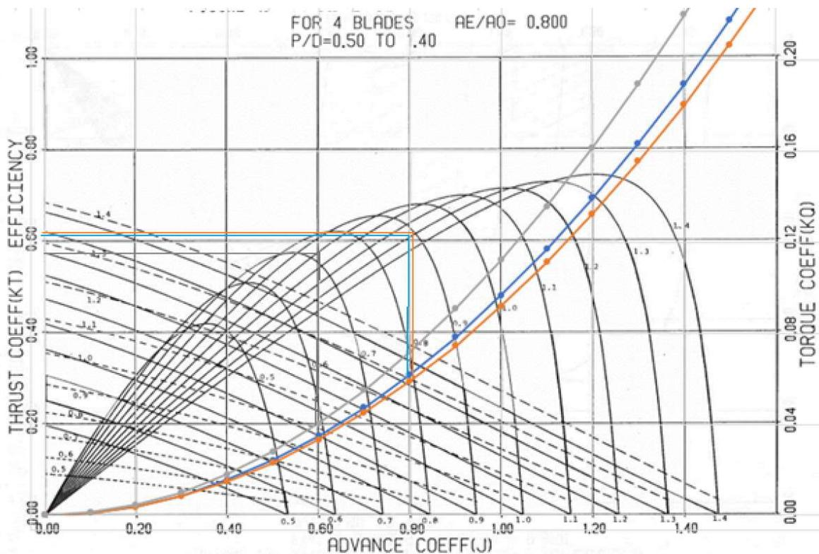
Figure 114: Open water Propeller diagram Wageningen B-series BAR=0.8, with graphed in KT lines <https://deepblue.lib.umich.edu/handle/2027.42/91702>
