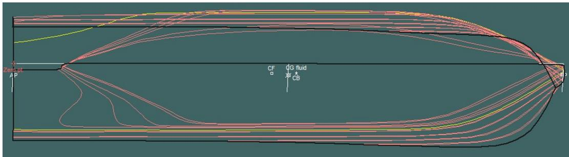
Figure 162: Water Lines at 10-degree heel
