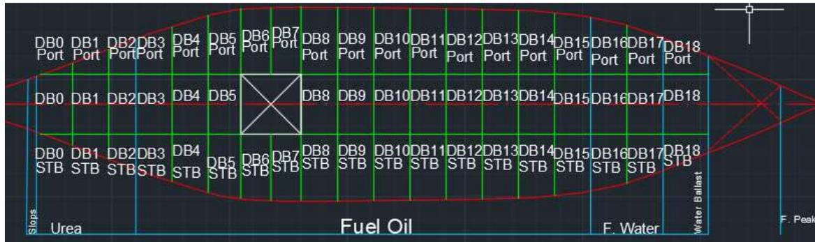
Figure 73: Tank Arrangement DB
