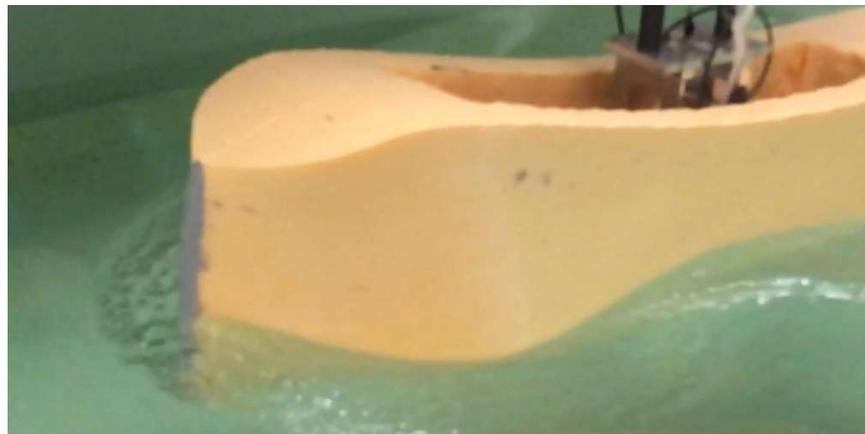
Figure 193: Bow Wave 14 kn
