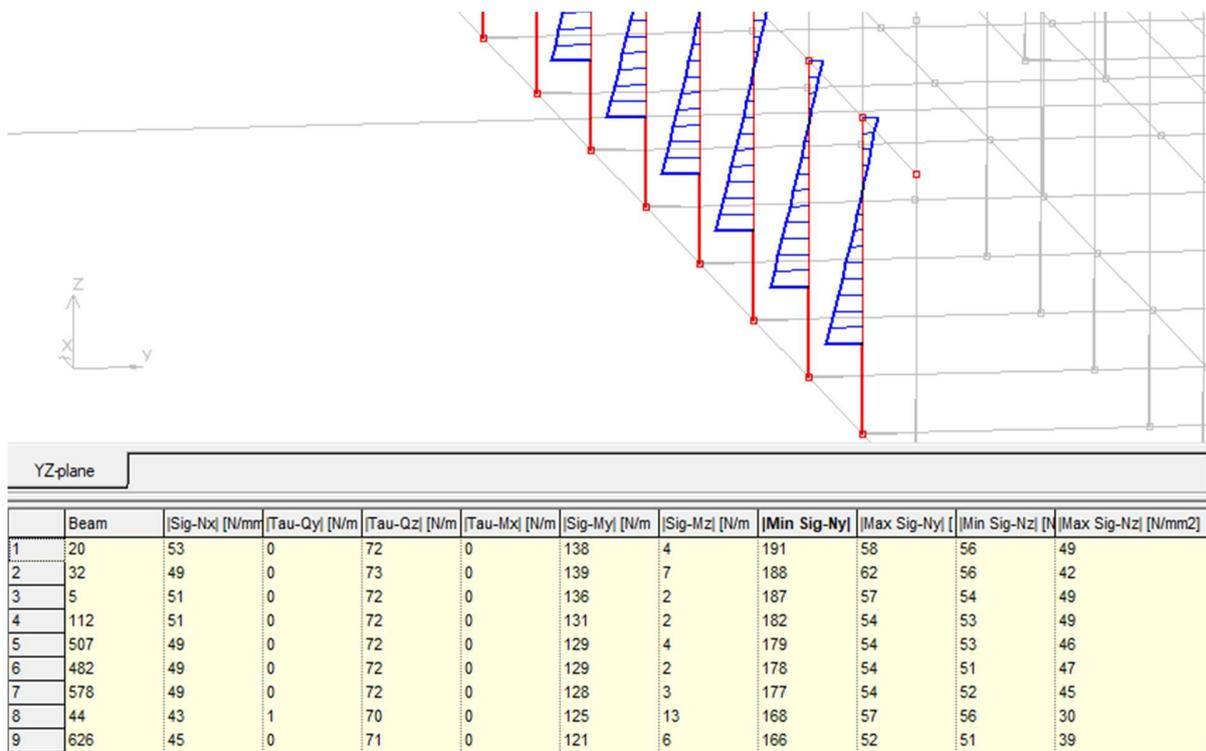
Figure 181 An example of a load-case without any load in the decks, resulting in excessive bending stresses.
