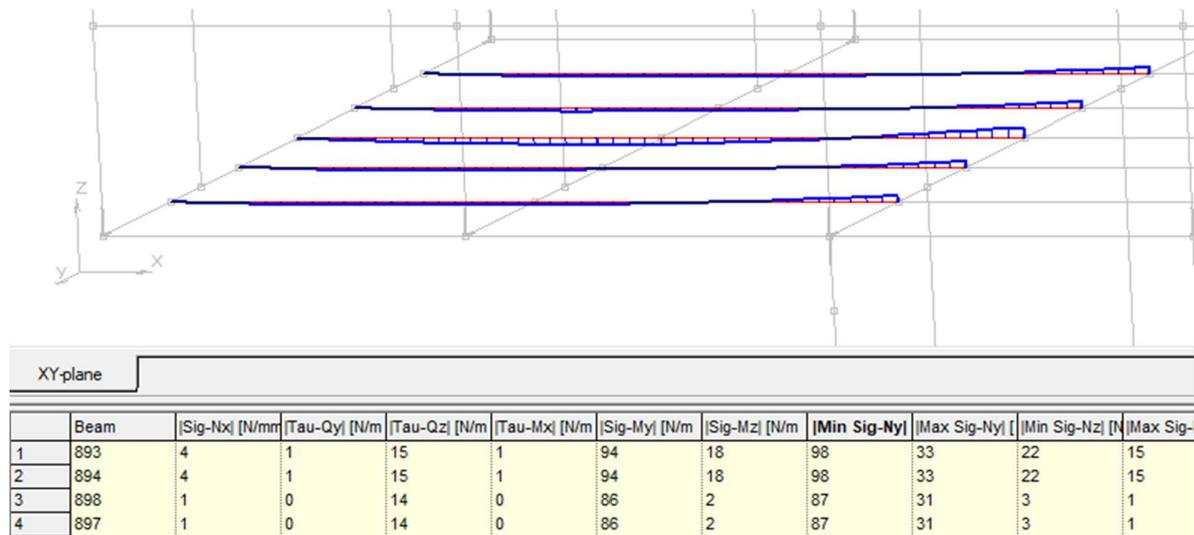
Figure 134 Bending moments and stresses on longitudinal members
