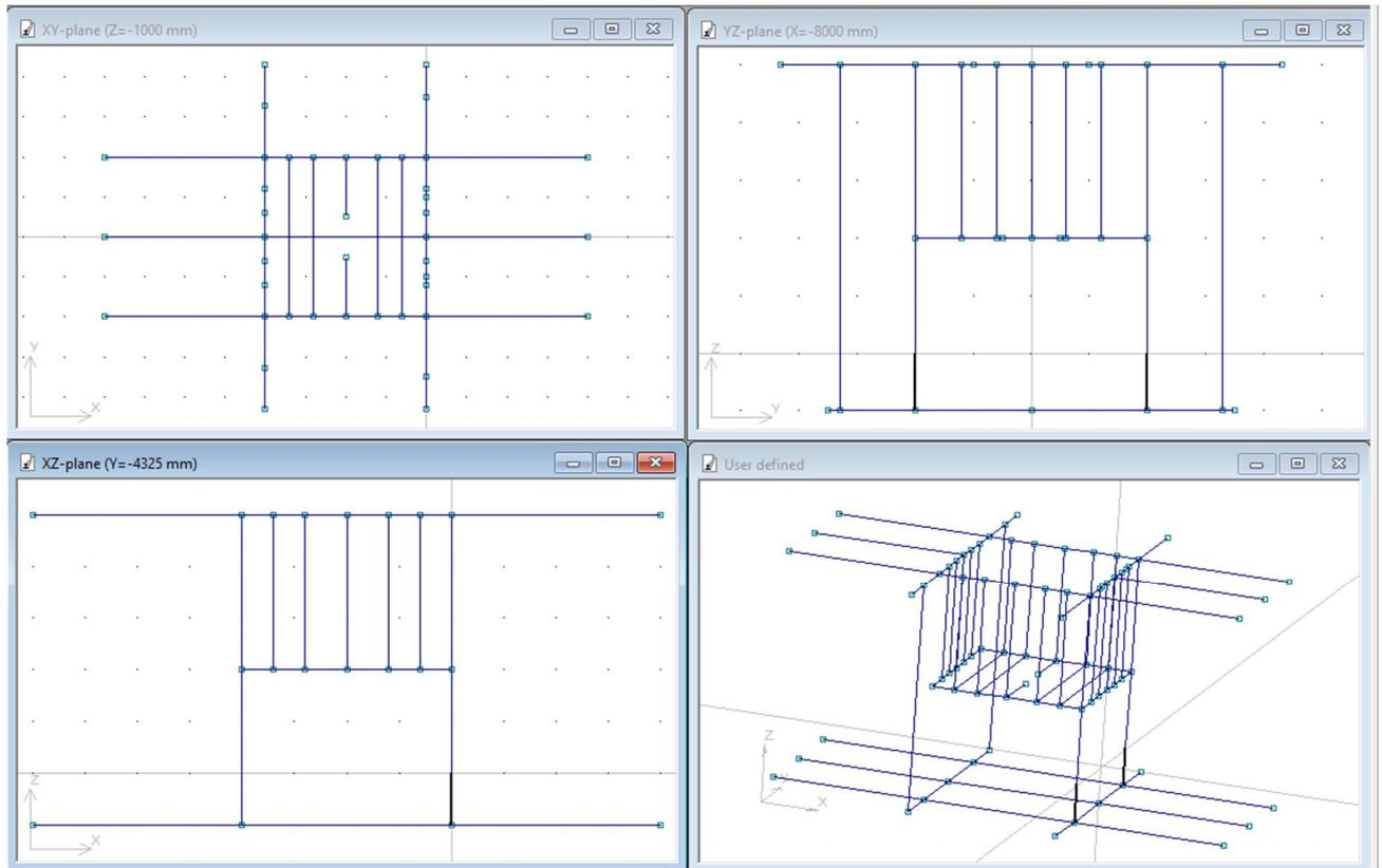
Figure 129 Moonpool structural arrangement in 3D-beam
