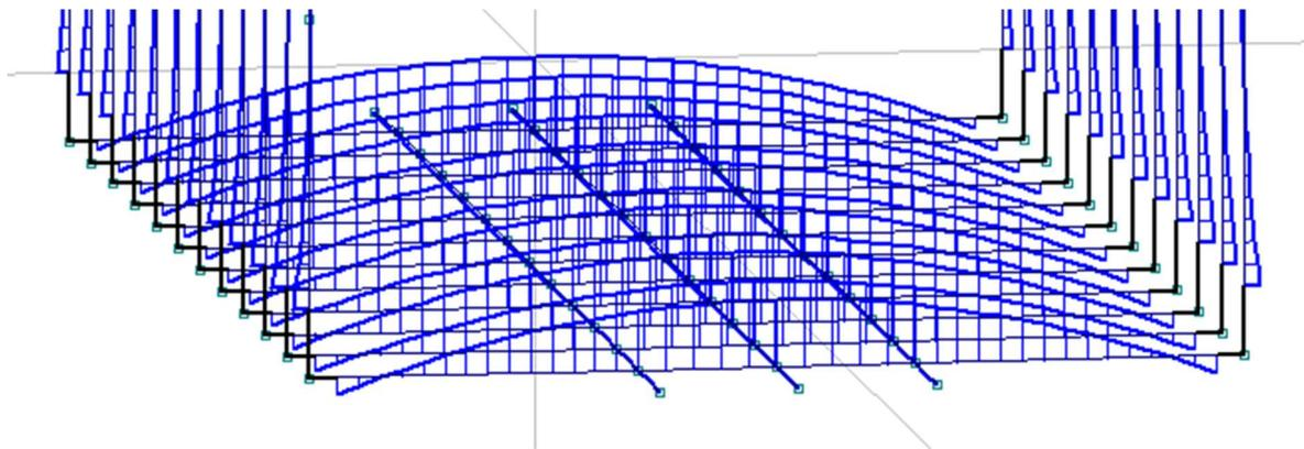
Figure 104 Bending-moments without a bulkhead
