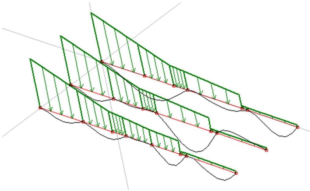
Figure 125 Stiffener supported by longitudinal girders hull side
