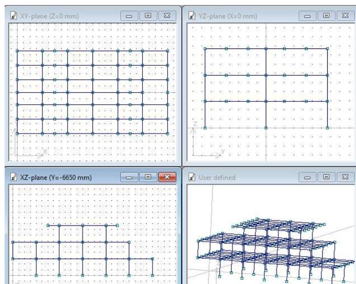
Figure 133 Structural arrangement of the accommodation with hatch in 3D-beam
