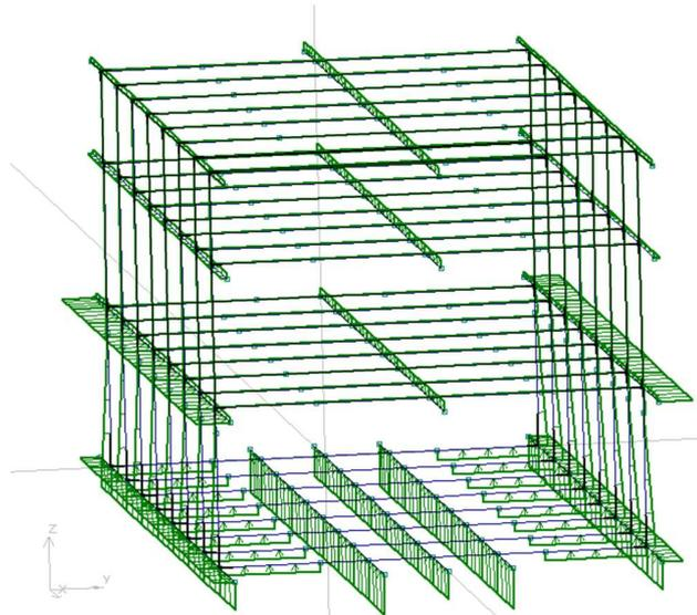
Figure 109 Applied load on transverse structure on 3D-Beam
