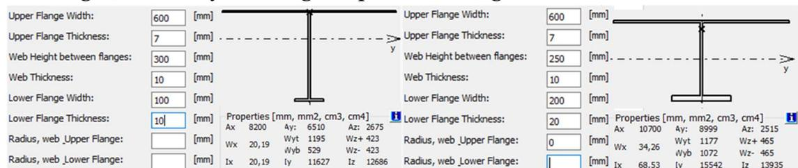
Figure 95 Comparing a high web vs a low web. Same section of modulus but different profile area.
