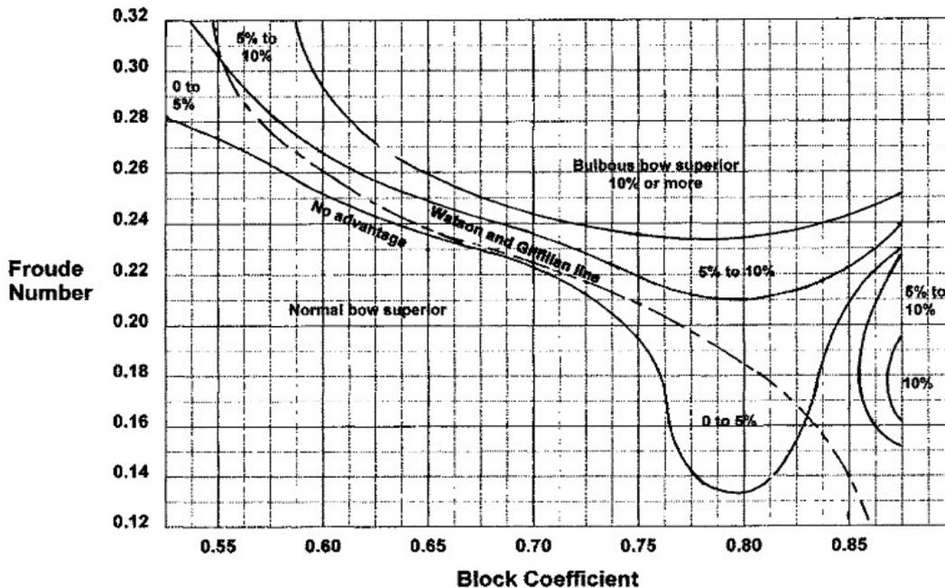
Figure 80- The Combination of Froude number and block coefficient at which bulbous bow are likely to be advantageous (Watson D. G., 1998)
