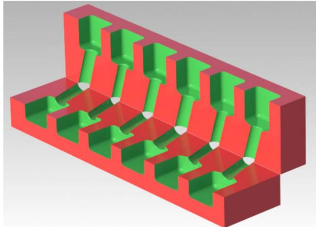
Figure 13 Moonpool model test with six designs
