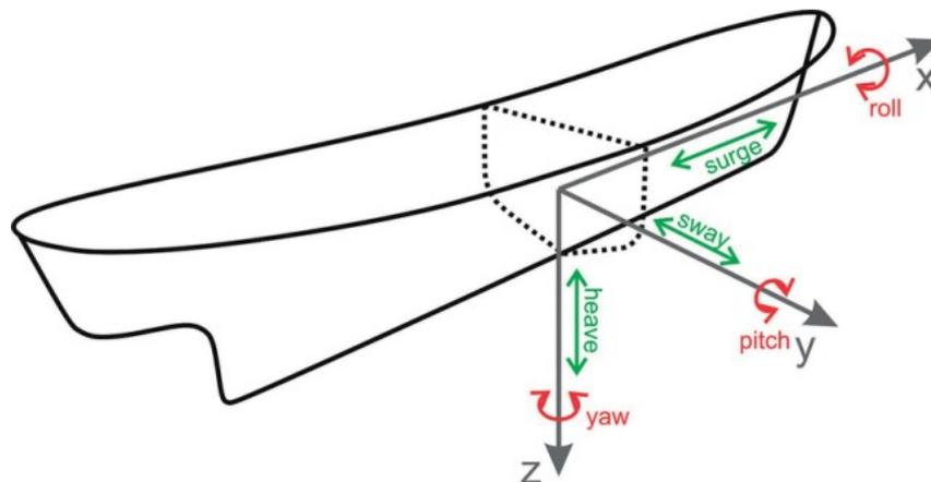
Figure 76 - Ship Motion; 6 Degrees of Freedom (DOF)
