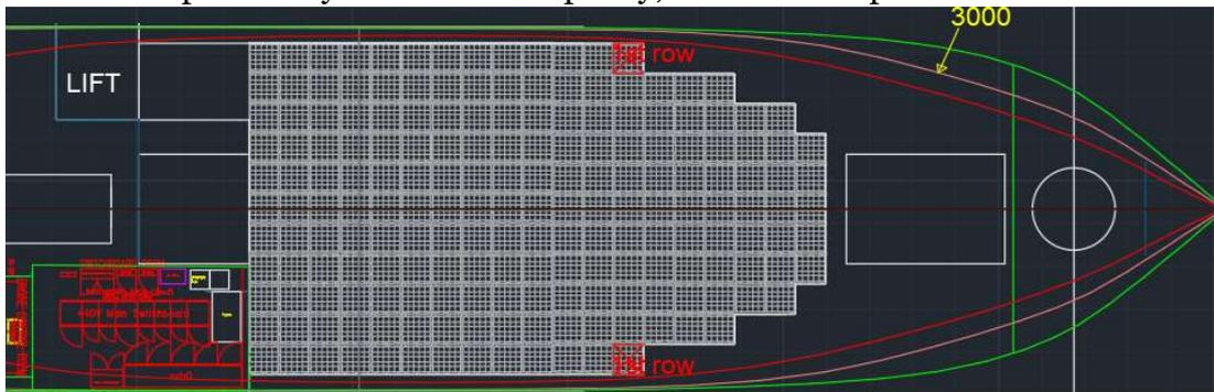
Figure 119: Pallet Arrangement 203
