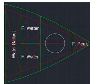
Figure 72: Tank Arrangement
