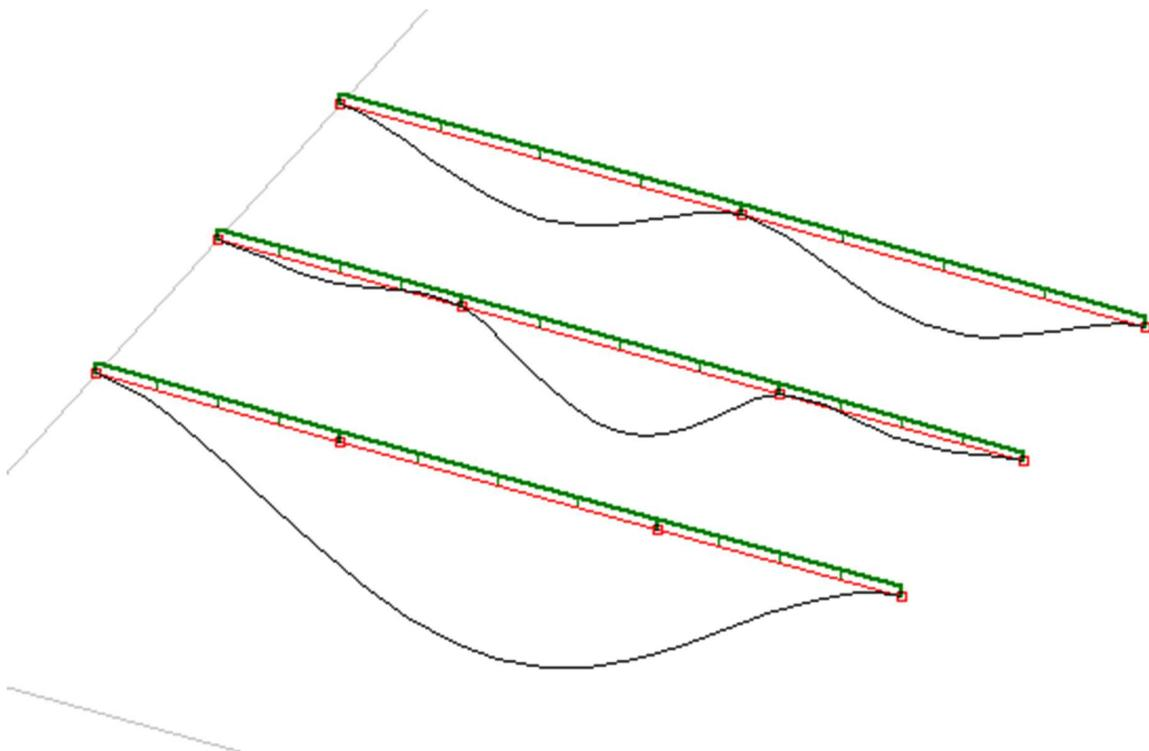
Figure 124 Stiffener supported by longitudinal girders decks
