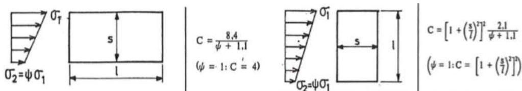
Figure 89 Buckling coefficient for pressure on the long side of the plate (Arne Jan Sollid, compendium, p.31)
