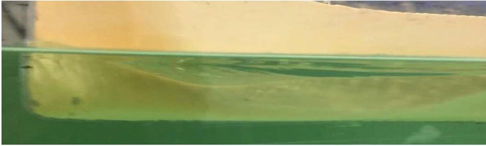
Figure 194: 14 kn Wave at Front Shoulder.
