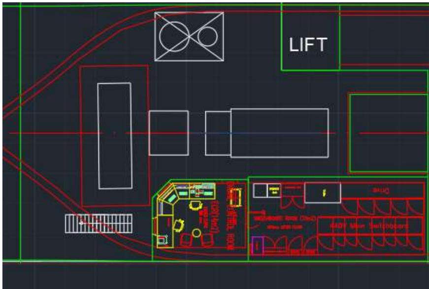
The Factory is moved 500 mm forward and the accommodations-rooms in front of the moonpool are moved 300 forward.
