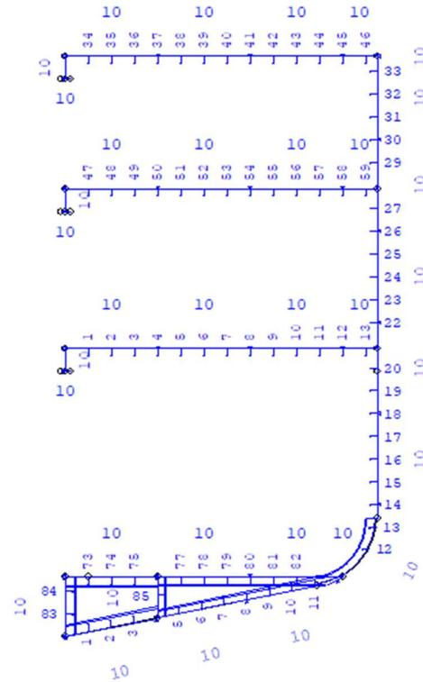
Figure 97 Sections scantling of the first structure
