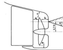
Fig. 2 Propeller clearances
