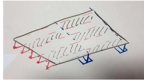
Figure 94 Stiffener and Girders creating rectangular plates
