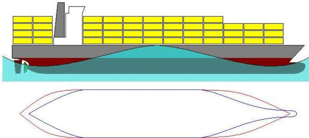
Figure 77 - Parametric Rolling
