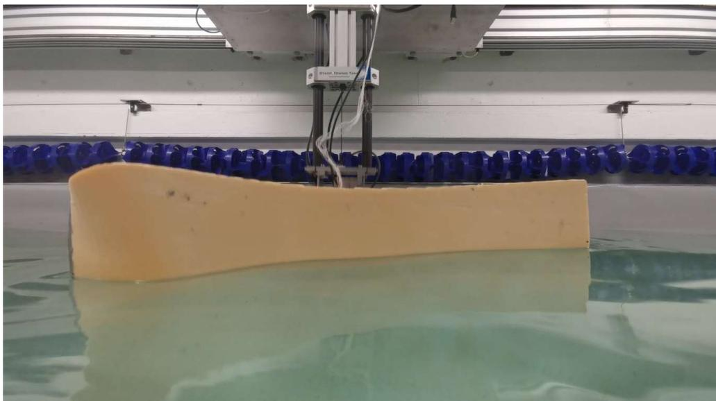
Figure 204: Stationary in waves, lowest draught Aft
