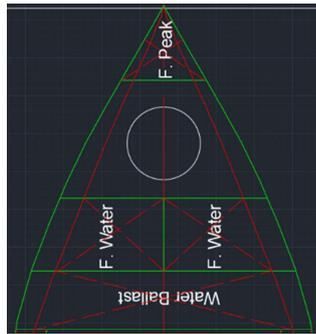
Figure 168: Tank Arrangement Bow over DB
