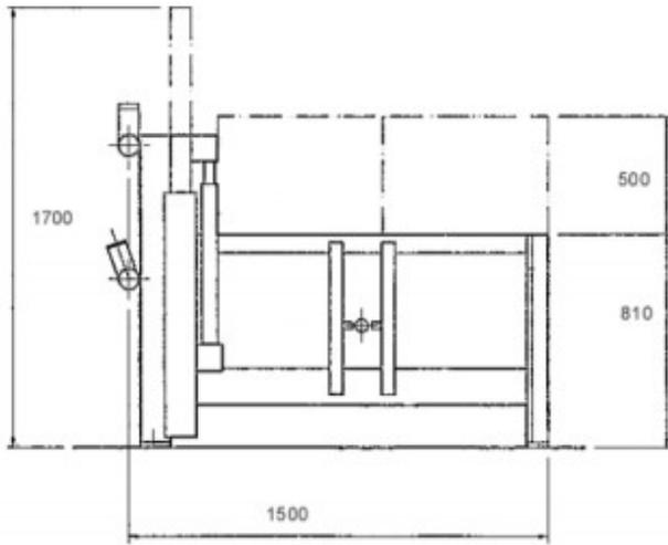
Figure 3 -Dimensions For Vertical Plate Freezer
