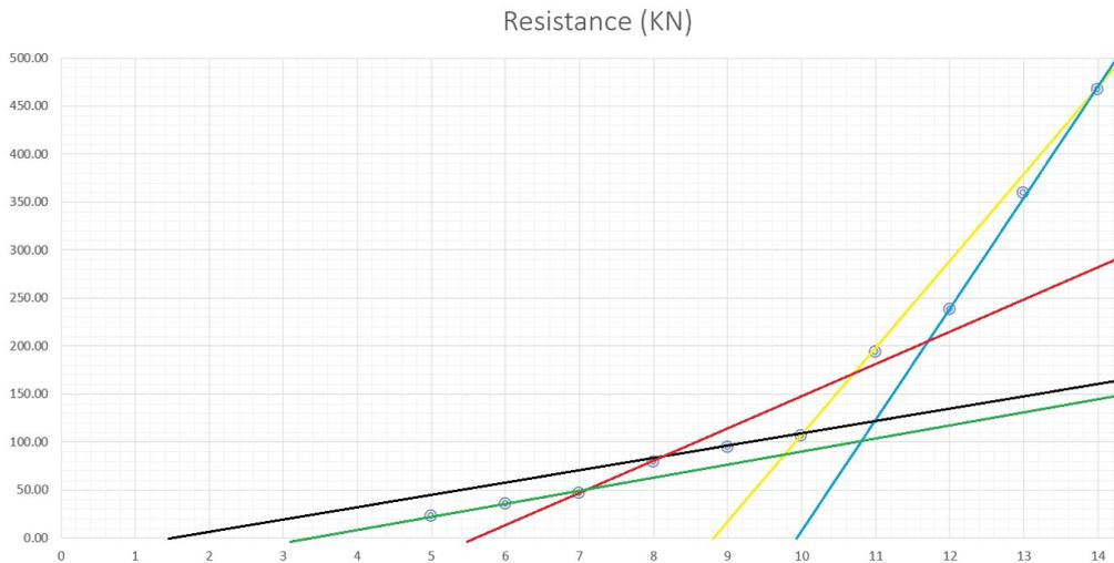
Figure 205: Analysis of Total Wave Resistance
