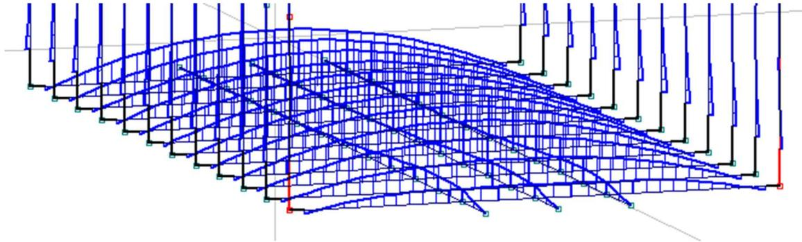
Figure 103 Bending moments with bulkhead in front
