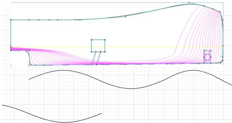
Figure 206 - Illustrating Efficiency Hump from Bow wave and Hollow from stern wave at 9 knots
