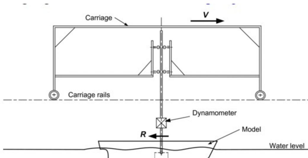
Figure 190: Towing Tank
