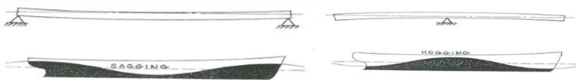
Figure 86 wave-moment sag (fig.42 link)
