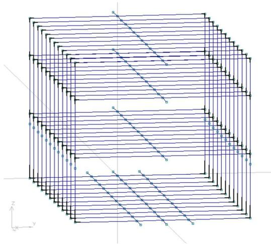
Figure 102 Longitudinal stiffened 3D beam structure
