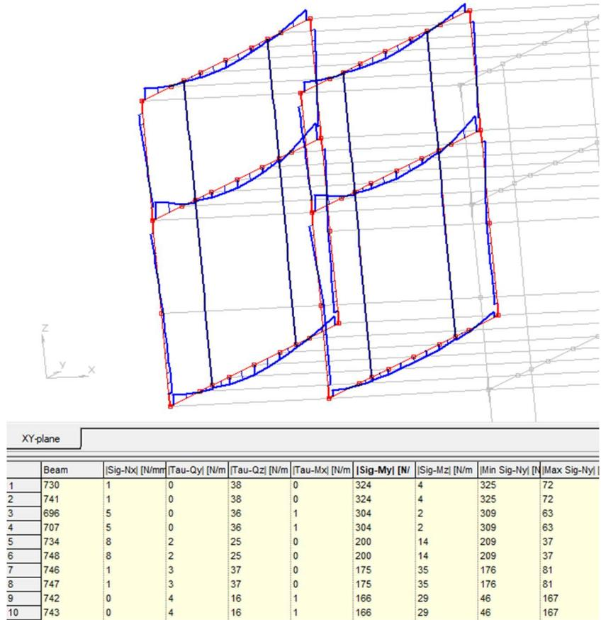
Figure 135 Bending-moments and stresses on transverse members
