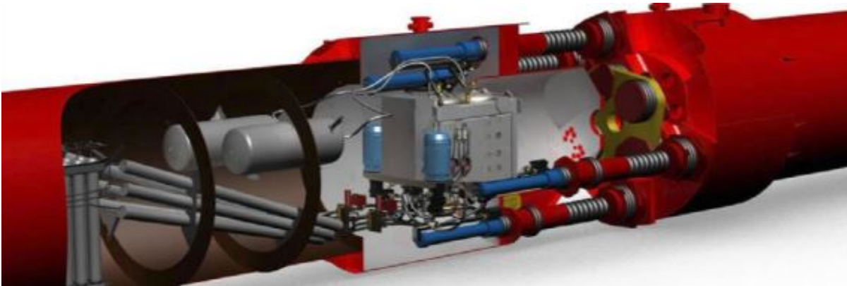
Figure 2.17: The joint and the PTO-system of Pelamis P2[8].
