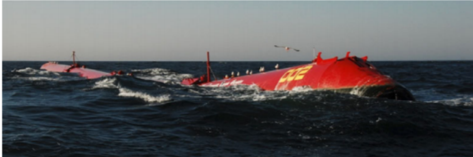
Figure 2.6: The Pelamis P1A-002 on site in Portugal[8].
