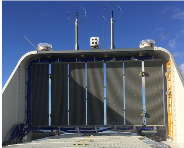
**Figure 3.1:** Two ultrasonic anemometers and LIDAR mounted on top of the nacelle. Picture by Lina Nordaune
