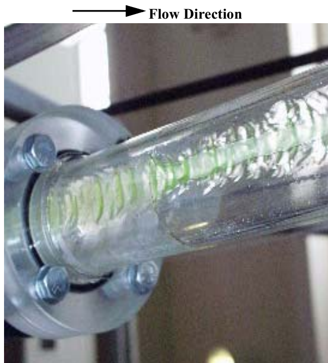
Figure 7-44: Picture taken from under the pipe of the water film contracting at the passage between a contaminated pipe wall (at the left) to a clean (pigged) pipe wall (at the right). This case is for input water fraction = 50%, superficial gas velocity = 10.5 m/s and superficial liquid velocity = 0.0059 m/s in the acrylic pipe
