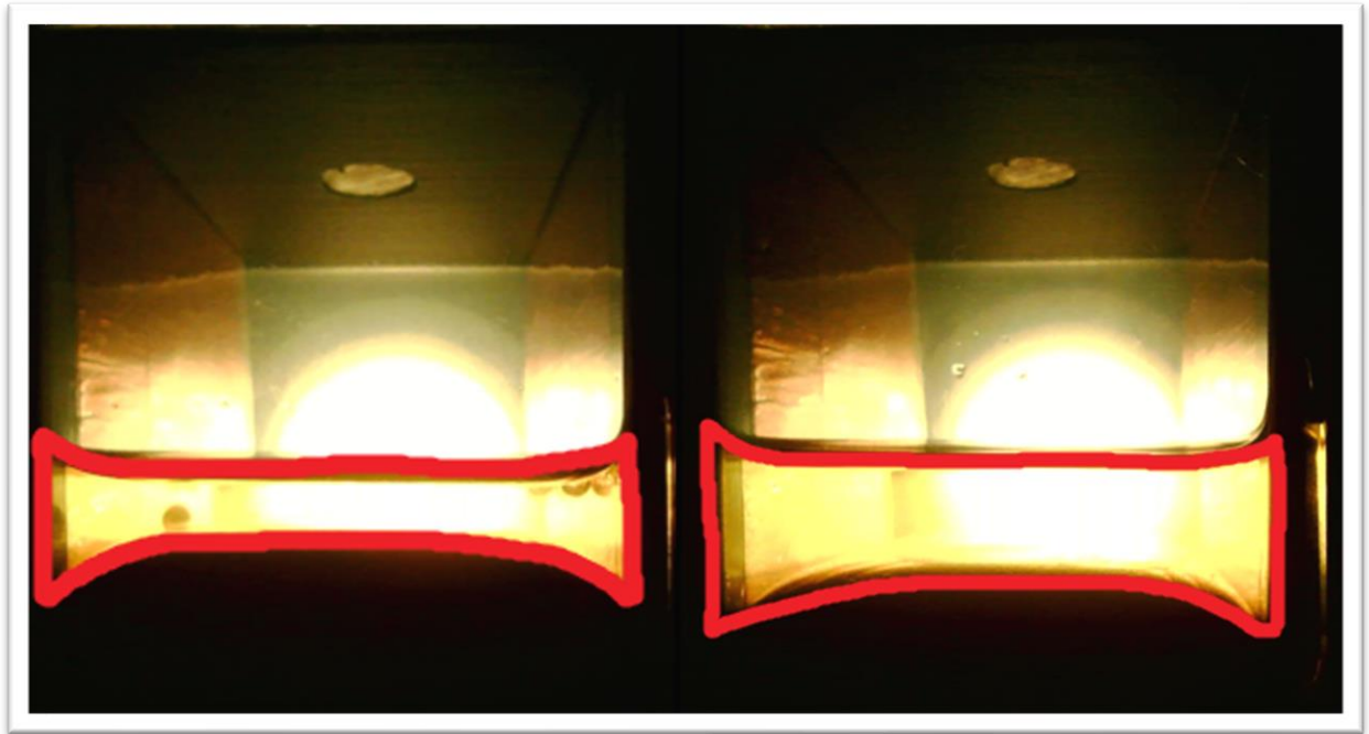
Figure 4.3 Area separated before and after electro coalescence.
