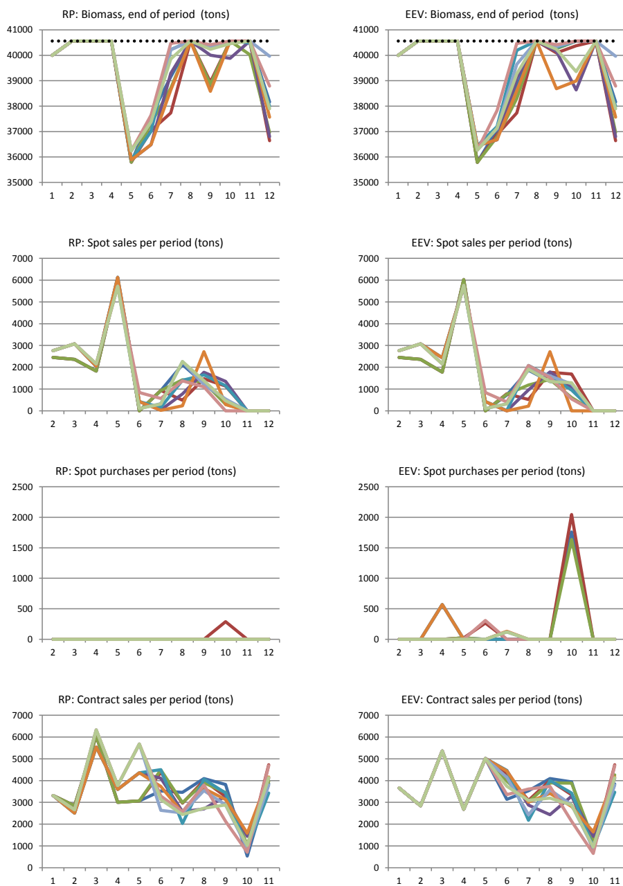
Figure 7.1: Detailed results for problem instance 1. The left column displays the details of the RP solution, the right column displays the details of the EEV solution. For all charts, periods are given on the x-axis, while the y-axis shows biomass in tons. The colored lines represent individual scenarios.
