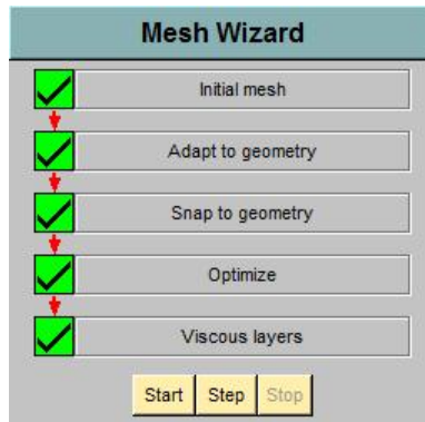
Figure 5.3: HEXPRESS grid generation interface
