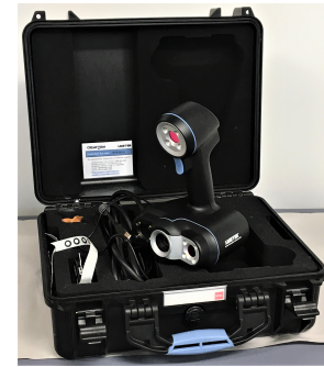
Figure 5.7: One of the laser scanner TOV uses for development and archiving casts is a Creaform GoScan! 50, an industrial 3D laser scanner.
