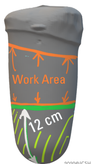
Figure 4.2: Preferred working area based on patient-Johns leg, drawn on a scanned model.
