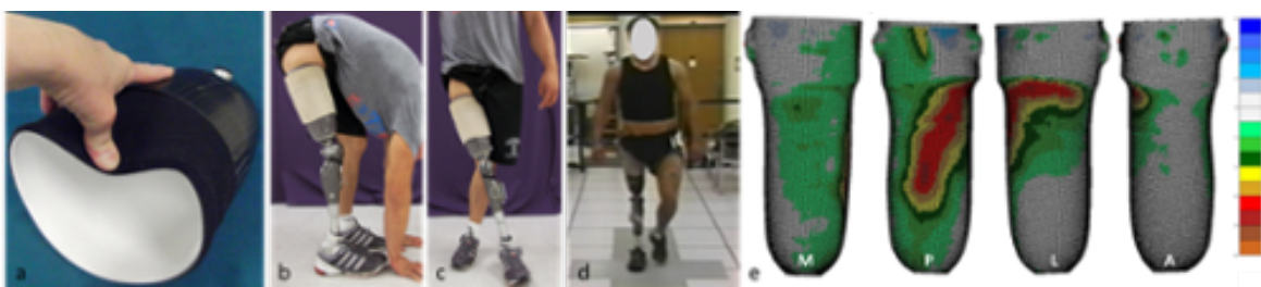
Figure 2.8: TOV uses the NU-FlexSIV method of Northwestern University to make subischial transfemoral prostheses. a) NU-FlexSIV Socket, b) and c) range of motion, d) Single limb stance stability, e) rectification map (from left: medial, posterior, lateral, anterior views) (Fatone, 2019)
