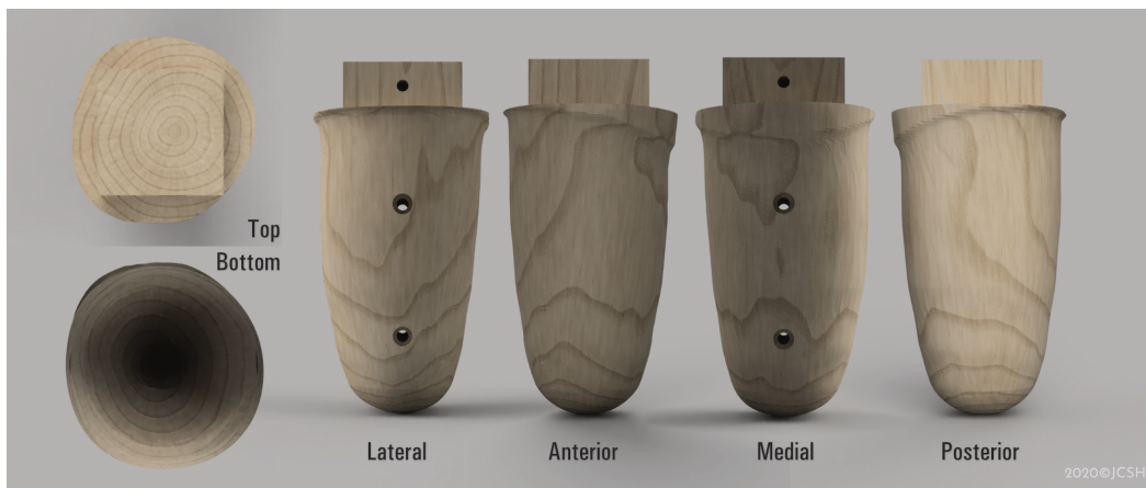
Figure 5.4: CAD Model of the stump after modification to remove the thickness of the liner from the stump. Views corresponding to Figure 5.3
