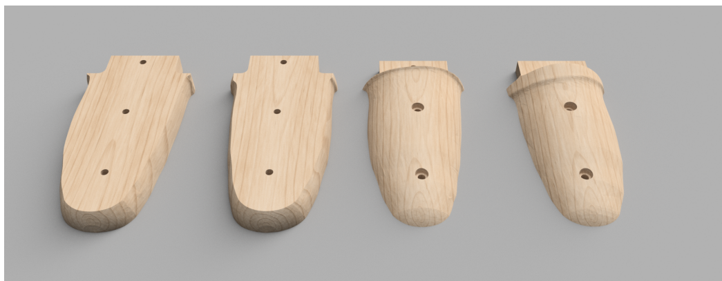
Figure 5.5: Stump model divided for milling. The two first were milled together in the first round and the two last in second round.
