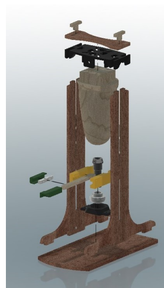
Figure 6.1: PD: CAD Test Rig Exploded View
