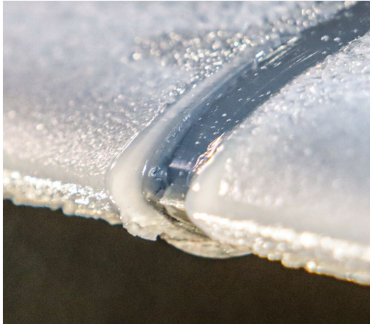
Figure 9.1: Chordwise cut into a 6min of ice accretion shows how the entire leading-edge is covered by ice.
