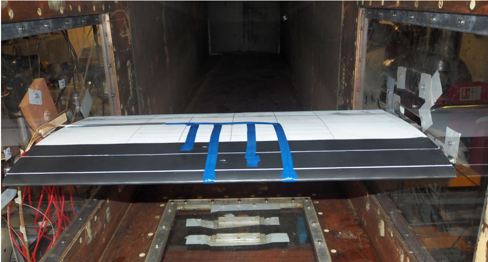
Figure 8.1: Ice protection system with five heating zones inside the wind tunnel. Four additional thermocouples have been added (blue tape).
