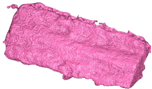
Figure 3.14: Photogrammetry result of a painted (dry) mixed ice segment that was carefully removed from the airfoil.
