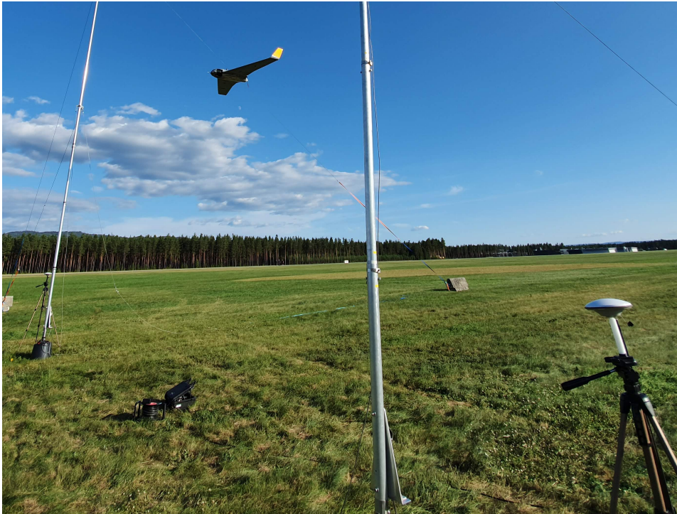
Figure 9.10: Picture of the UAV flying through the net rig, without a physical net. The GNSS-antennas are mounted on tripods on each side of the net, while the net instrumentation suitcase is in the center.
