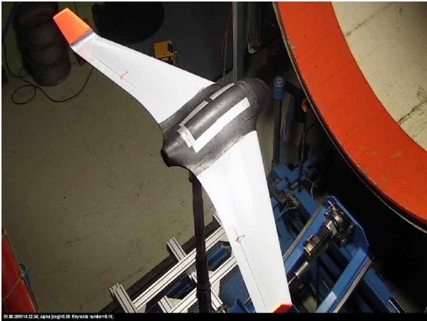
Figure 4.1: The Skywalker X8 mounted in the wind tunnel
