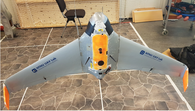
Figure 6.1: The Skywalker X8 mounted to oscillate around its x-axis as a bifilar pendulum
