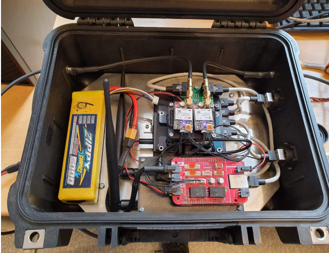
Figure 9.7: Picture of the instrumented net suitcase, showing the two GNSS receivers on top of the SenTiBoard and an ethernet switch. In the front is the onboard computer with a custom cape, on top of the 5 GHz radio.
