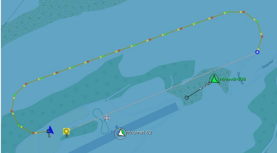
Figure 9.3: The recovery plan generation GUI, with the start (blue), the arrest system (white), the UAV (green) and the plan inbetween. The small black circle ahead of the UAV corresponds to the carrot point, while the dynamic plan is not in the map view.
