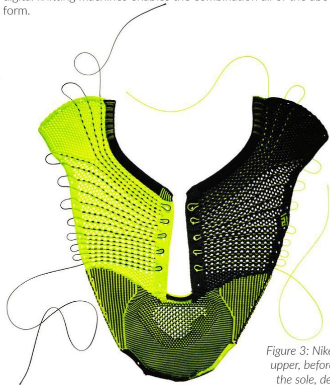
Figure 3: Nike's 3D knitted upper, before assembly to the sole, demonstrates a combination of mechanically varying structures knitted seamlessly in one piece.
